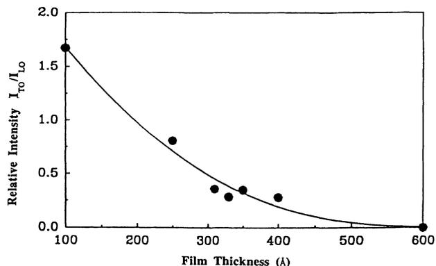
FIG. 8. Thickness dependence of the ratio of the TO intensity to the LO intensity. The solid line is only a guide to the eyes.
