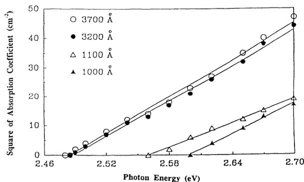
FIG. 7. Square of the absorption coefficient of CdS thin films plotted against the photon energy.
