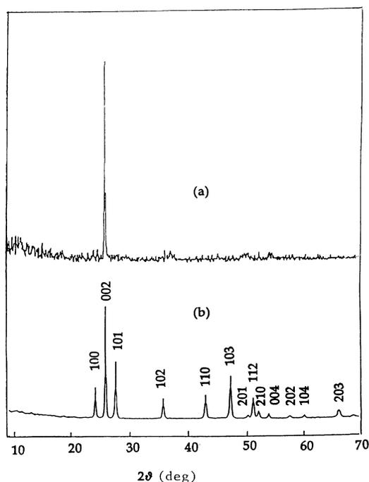
FIG. 1. (a) The XRD spectrum of the as-deposited CdS films on silicon substrate at room temperature. (b) The pattern of CdS powders.
