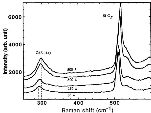
FIG. 3. Thickness dependence of the 1LO phonon energies. These RRS spectra of CdS films deposited on a *p*-type silicon wafer were excited at 4880 Å and were detected at room temperature. CdS film thickness is indicated in the figure. The dashed line marks the frequency of the main Raman peak (300  $\text{cm}^{-1}$ ) for a thick (800 Å) film.
