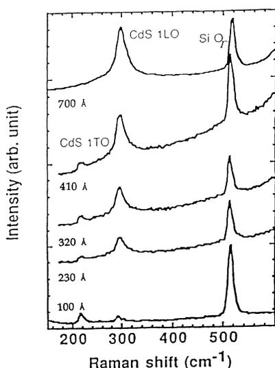
FIG. 5. Thickness dependence of the 1TO phonon intensities and energies. The RRS spectra of CdS films deposited on the *p*-type (100) silicon wafer were detected at room temperature. The spectra were excited at  $4880\text{ \AA}$ .
