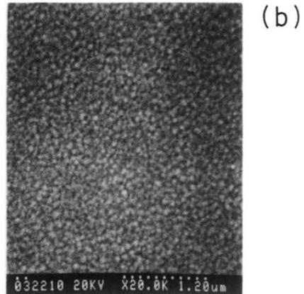
FIG. 2. The SEM photographs for the films grown on silicon substrates at temperature (a) 30°C and (b) 100°C.
