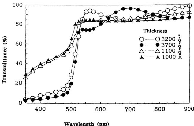
FIG. 6. Spectral dependence of the transmittance for the as-deposited films deposited on glass substrate at different thickness.
