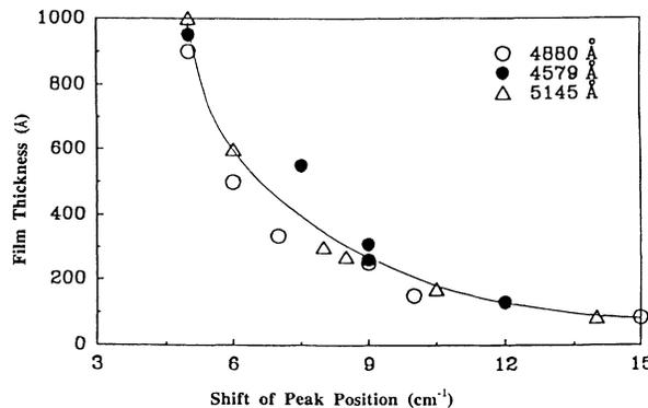
FIG. 4. Frequency downshifts of the 1LO Raman peaks relative to its position for bulk CdS as a function of film thicknesses. The full curve is drawn to guide the eye. The Raman spectra were excited at 4579, 4880, and 5145 Å.
