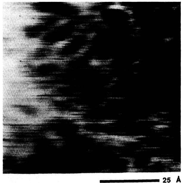
FIG. 2. STM image of the contaminated K_{0.30}MoO_3 surface at 143 K.
