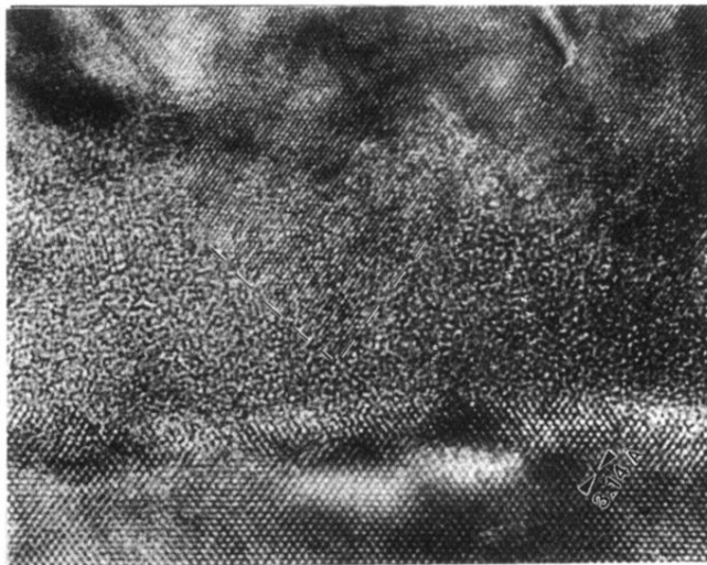
FIG. 15. High-magnification high-resolution XTEM micrograph showing an amorphous interfacial layer between the diamond and silicon substrates.
