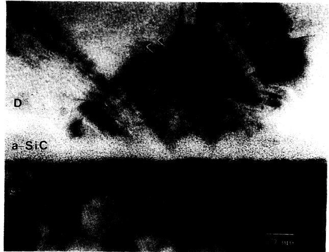
FIG. 14. Low-magnification high-resolution XTEM micrograph showing several nucleation sites and an interfacial layer between silicon and diamond.
