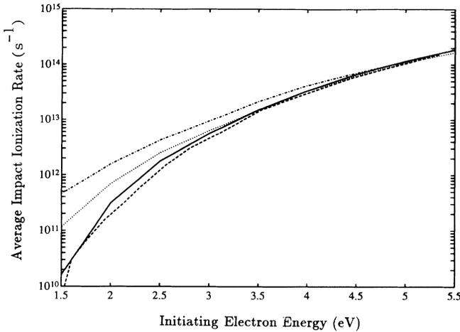
FIG. 1. Impact ionization rates for Si averaged over all initial electron states with a given energy measured from the bottom of the conduction band. Dashed curve, Kane's result; solid curve, zero-field, no collision broadening; dotted curve, collision broadening; dash-dotted curve,  $F=5 \times 10^5$  V/cm and collision broadening.
