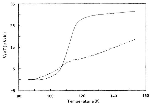
FIG. 3. The temperature dependence of  $V_R/\Delta T + S$  and  $V_R/\Delta T - S$ . The former is represented by a solid line and the latter by the dashed line.
