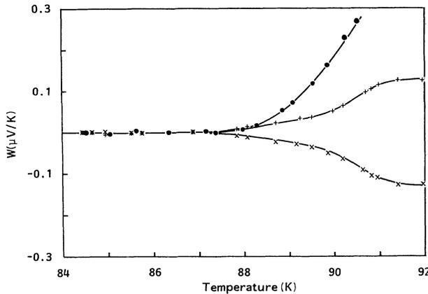
FIG. 4. The temperature dependence of  $W_A \equiv V_R/\Delta T - S$ ,  $W_B \equiv -V_R/\Delta T - S$ , and  $W_C \equiv V_R/\Delta T + S$  are labeled by  $\bullet$ ,  $+$ , and  $\times$ , respectively. The solid lines are guides for the eye. Note that  $S$  starts to deviate from zero at  $T \approx 87.3$  K, whereas the resistive component  $V_R/\Delta T$  only becomes nonzero at a higher temperature,  $T \approx 88.3$  K.
