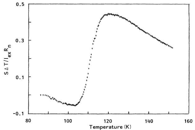
FIG. 2. The ratio of the thermoelectrically generated supercurrent ( $I_s = S\Delta T/R_n$ ) to the external applied current ( $I_{\text{ex}}$ ).
