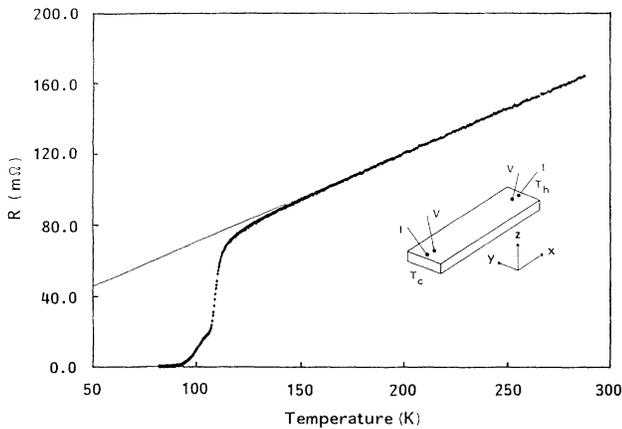
FIG. 1. Resistance  $R = R(T)$  of the sample at an excitation current density of  $0.1 \text{ A/cm}^2$ . The inset shows the sample geometry and contact configuration used in this study. The straight line represents the normal resistance  $R_n(T)$  extrapolated from  $T > 220 \text{ K}$ .  $T_c$  and  $T_h$  represent the temperatures of the cold and hot ends, respectively, of the sample as measured by two calibrated PT100 platinum thermometers.
