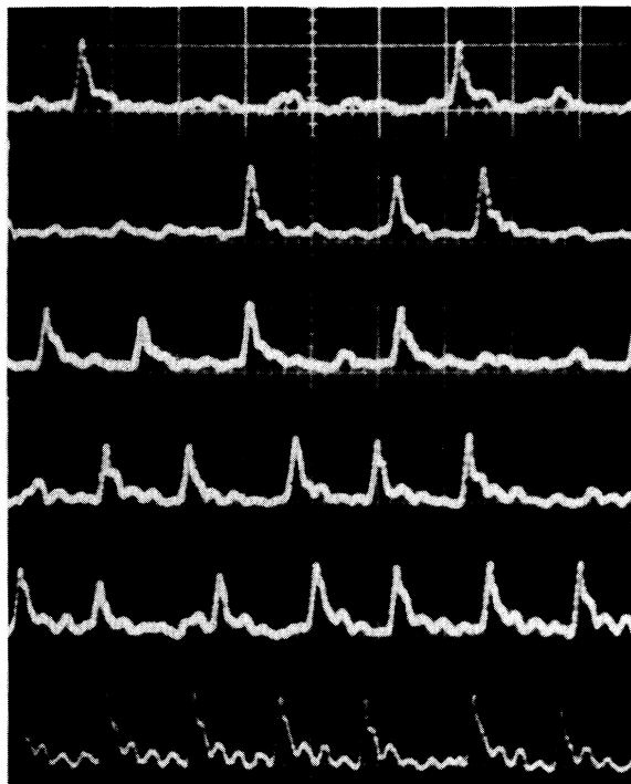
FIG. 6. Oscilloscope traces of the auto-oscillation obtained with subsidiary-resonance pumping with increasing microwave field R = h/h'_c in a YIG sphere oriented along [110], H_0 = 1950 Oe, f_p = 9.4 GHz. The time scale is 10 \mu\text{s} per division. R = 1.862, 1.872, 1.883, 1.894, 1.905, and 1.916 from top to bottom. Note that the auto-oscillation sets in with a finite amplitude and rapidly increasing frequency, quite differently from the Hopf scenario of Fig. 4.
