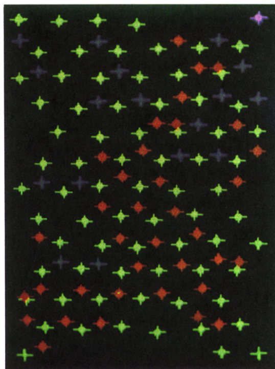
FIG. 8. A photograph of (part of) the same configuration as illustrated in Fig. 7. Included is a projection of the central (110) plane of I^- ions (light green) and those Ag^+ ions which are found within a rectangular slab which contains this central plane. The only Ag^+ ions found are of type 4 (red) and type 3 (blue)—which occur in nonoverlapping regions.
