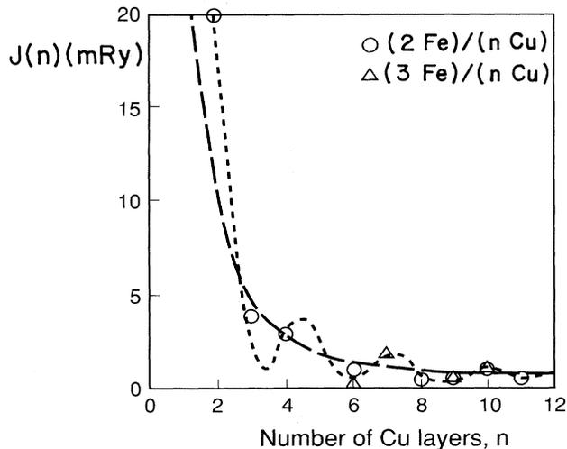
FIG. 4. Calculated exchange interaction energy  $J(n)$  (per antiferromagnetic unit cell) for bcc Fe/Cu(100) superlattices, as a function of the Cu layer thickness  $n$ , after Herman *et al.*<sup>18</sup> Circles and triangles refer to Fe layers composed of 2 and 3 Fe monolayers, respectively. The broken and dotted curves are explained in the text.
