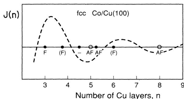
FIG. 3. Analysis of experimental data on the exchange interaction across Cu layers in fcc Co/Cu(100) systems, in terms of an oscillatory interaction function  $J(n)$ . Open circles: Ref. 5; closed circles: Ref. 6. F, AF, and – denote ferromagnetic, antiferromagnetic, and no (experimentally detectable) coupling, respectively. Parentheses denote that the coupling is relatively weak.
