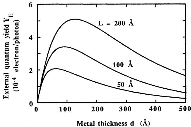
FIG. 1. Front illumination external quantum yield  $Y_E$  of Schottky diodes calculated as a function of metal thickness  $d$ . The photon energy is 1 eV, the Fermi energy  $E_F$  is taken as equal to 3.5 eV, the Schottky barrier height  $\phi$  is 0.64 eV, the metal indices are  $n=1$  and  $k=5.4$ , and the calculation has been carried out for three values of escape depth  $L$ , 50, 100, and 200 Å.
