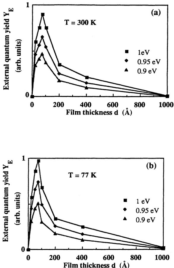
FIG. 2. Experimental external quantum yield or photocurrent per incident photon measured in CoSi<sub>2</sub> Schottky diodes at 300 K (a) and at 77 K (b) as a function of metal thickness  $d$ . The results are presented for three different photon energies: 1, 0.95, and 0.9 eV. The photocurrent is given here in arbitrary units, with the same numerical factor for both (a) and (b), so that the photocurrent values of both figures can be compared.
