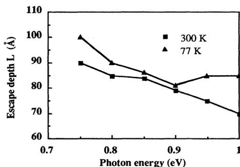
FIG. 3. Hot-electron escape depth  $L$  in CoSi<sub>2</sub> deduced from photocurrent measurements in Schottky diodes as a function of photon energy. The results are given in 300 and 77 K, with an accuracy of the order of 20 Å.
