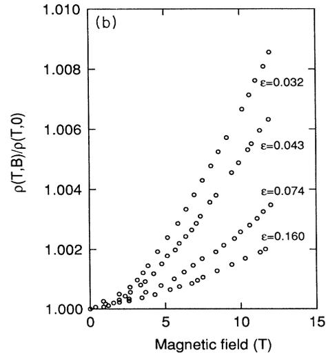
FIG. 2. Relative magnetoresistivity for  $\text{YBa}_2\text{Cu}_3\text{O}_{7-\delta}$  in magnetic fields up to 12 T and temperatures ranging from 92.79 K [ $\epsilon = (T - T_c)/T_c = 0.07$ ] to 106.88 K ( $\epsilon = 0.160$ ). Note the different scales for  $\Delta\rho/\rho$ . For clarity, all curves used in the analysis are not shown in the figure.
