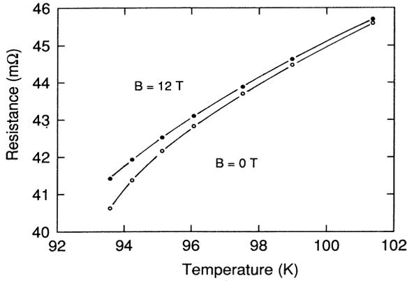
FIG. 1. Sample resistance vs temperature at zero magnetic field and at a magnetic field of 12 T for temperatures above the superconducting transition temperature,  $T_c = 92.16$  K.
