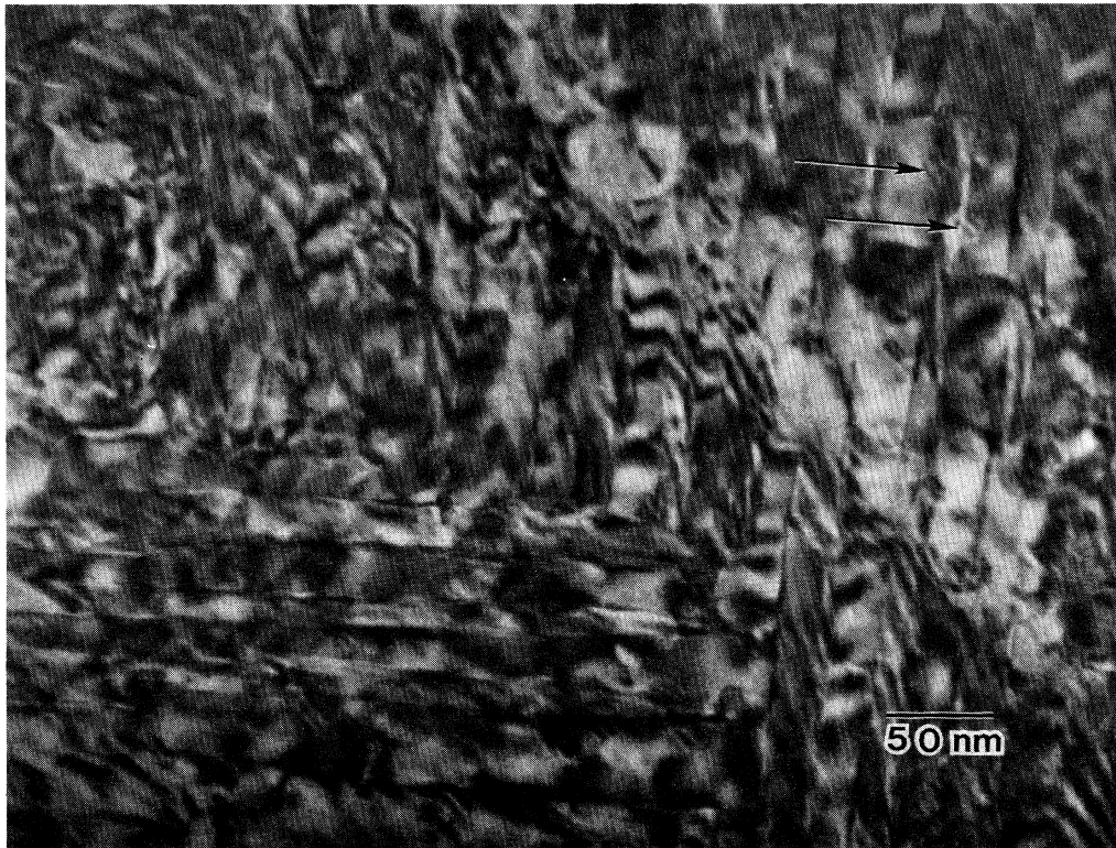
FIG. 9. Bright-field electron micrograph of a planar section of \text{YBa}_2\text{Cu}_3\text{O}_x on \text{SrTiO}_3 showing a twinned structure. Some a -axis grains are indicated by arrows.
