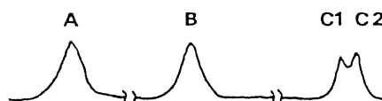
FIG. 6. Typical cw-NMR spectrum for a sample with a multipeak structure, C1 and C2, besides the usual A and B domain signals.
