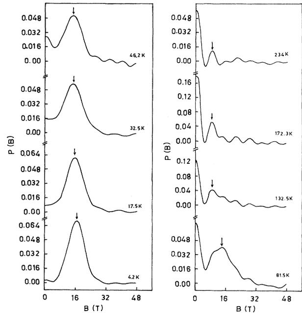
FIG. 2. The probability,  $P(B)$ , of the hyperfine field ( $B$ ) obtained at different temperatures for the Mössbauer spectra of Fig. 1.
