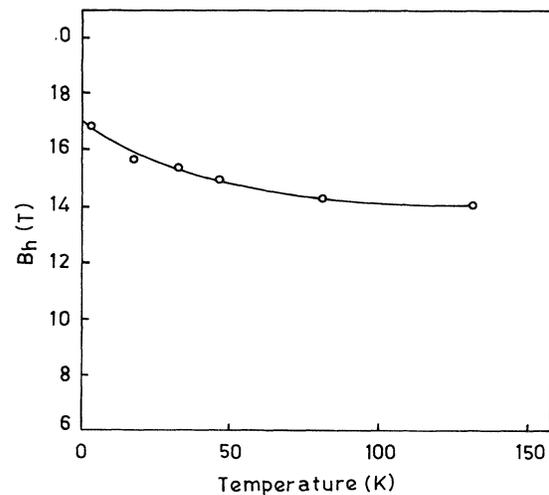
FIG. 3. The value of hyperfine field ( $B_h$ ) corresponding to the high-field peak (indicated by arrows in Fig. 2) plotted as a function of temperature.
