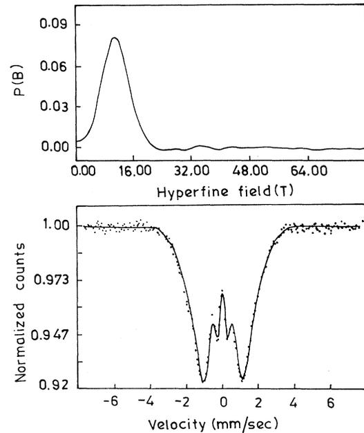
FIG. 6. The Mössbauer spectrum for  $\text{Cr}_{74}\text{Fe}_{26}$  in an externally applied field of 5 T in a direction perpendicular to the direction of  $\gamma$  transmission, and the corresponding field distribution.
