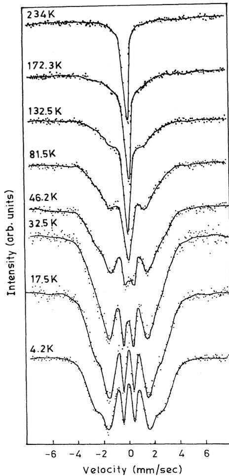
FIG. 1.  $^{57}\text{Fe}$  Mössbauer spectra of the  $\text{Cr}_{74}\text{Fe}_{26}$  alloy at different temperatures recorded in the transmission geometry. The solid lines through data are obtained by a model-independent field-distribution fit.
