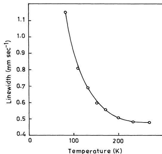
FIG. 7. The experimental linewidth of Mössbauer spectra plotted as a function of temperature.
