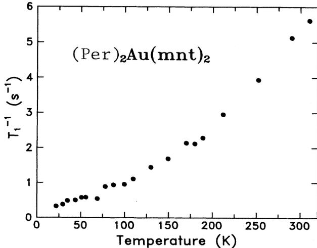
FIG. 5. Temperature dependence of  $^1\text{H}$  nuclear-spin-lattice relaxation rate ( $T_1^{-1}$ ) for  $(\text{Per})_2[\text{Au}(\text{mnt})_2]$ . Note the upwards deviation to the Korringa law ( $T_1^{-1} \propto T$ ).
