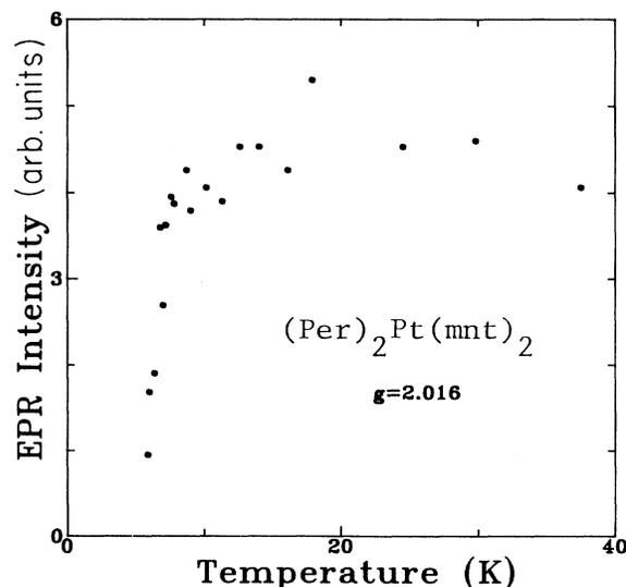
FIG. 6. The integrated intensity of EPR signal for  $(\text{Per})_2[\text{Pt}(\text{mnt})_2]$ , after Ref. 5.
