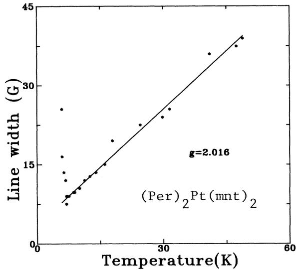
FIG. 7. EPR linewidth as a function of emperature for  $(\text{Per})_2[\text{Pt}(\text{mnt})_2]$ , after Ref. 5.
