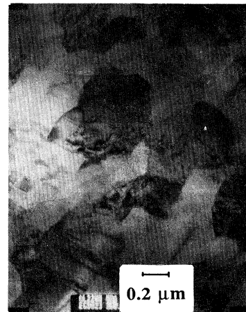
FIG. 3. Microstructure of decagonal T\text{-Al}_{78}\text{Mn}_{22} phase observed by transmission electron microscopy.
