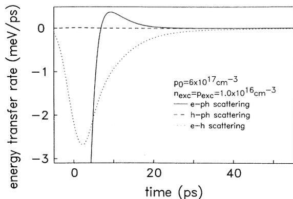
FIG. 3. Energy-loss rates of the carriers in a  $p$ -doped sample as a function of the delay time. Shown are the energy loss of the electrons (solid line) and holes (dashed line) due to scattering with phonons and the energy exchange between electron and holes due to Coulomb scattering (dotted line).
