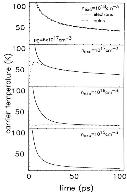
FIG. 2. Cooling curves calculated for a *p*-doped sample with a doping density of  $6 \times 10^{17} \text{ cm}^{-3}$  and various excitation densities. The electron and hole temperatures are the solid and dashed lines, respectively.
