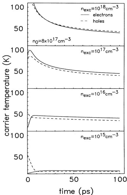
FIG. 1. Cooling curves calculated for an *n*-doped sample with a doping density of  $8 \times 10^{17} \text{ cm}^{-3}$  and various excitation densities. The lattice temperature is set to 4 K. The electron and hole temperatures are the solid and dashed lines, respectively.
