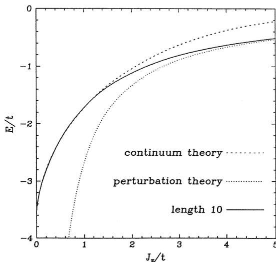
FIG. 3. Ground-state energy of the  $t$ - $J_z$  model compared to large- $J_z$  perturbation theory and the continuum theory (Ref. 10).
