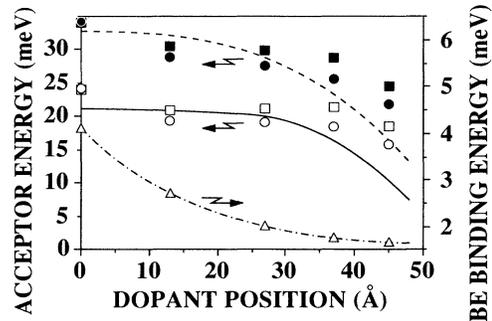
FIG. 2. BE binding energy, represented by open triangles vs the dopant position  $z_0$  in the well for the samples used in the study. The dash-dotted line is a fit to the experimental data. The upper set of data corresponds to the  $1s \rightarrow 2s$  acceptor transition energies and the total acceptor binding energies vs the dopant position  $z_0$  in the well. The squares are from THT data and the circles are from RRS data.
