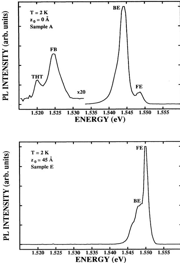
FIG. 1. PL spectra for (a) sample *A* ( $z_0=0 \text{ \AA}$ ) and (b) sample *E* ( $z_0=45 \text{ \AA}$ ) using a  $\text{Kr}^+$  ion laser as an excitation source.
