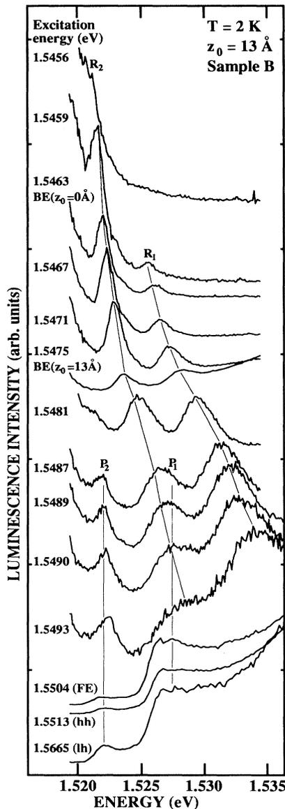
FIG. 3. SPL spectra of sample  $B$  ( $z_0 = 13 \text{ \AA}$ ) using an excitation intensity of  $\approx 100 \text{ mW/mm}^2$ . The notations (hh) and (lh) denote the heavy-hole and light-hole states of the FE as observed in PLE, and (FE), [BE ( $z_0 = 13 \text{ \AA}$ )], and [BE ( $z_0 = 0 \text{ \AA}$ )] denote the FE and the BE, bound to acceptors at  $z_0 = 13 \text{ \AA}$  and at the center of the well ( $z_0 = 0 \text{ \AA}$ ), respectively, as observed in PL.
