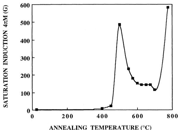
FIG. 1. Room-temperature saturation induction  $4\pi M$  vs annealing temperature  $T_a$  data for a sample of rf-sputtered amorphous  $(1-2x)\text{BiFeO}_3-x\text{ZnFe}_2\text{O}_4$  with  $x=0.125$  for an in-plane static field of 5 kOe. The sample was sputtered in 50% oxygen and 50% argon atmosphere and the annealing was performed at  $T_a$  in air for 60 min.
