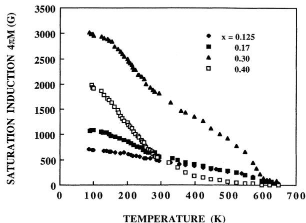
FIG. 4. Saturation induction vs temperature data for samples of  $(1-2x)\text{BiFeO}_3-x\text{ZnFe}_2\text{O}_4$  annealed at  $650$ – $700^\circ\text{C}$ .
