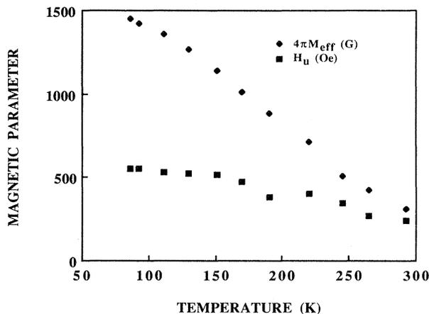
FIG. 6. Variation of the effective magnetization  $4\pi M_{\text{eff}}$  with temperature obtained from ferromagnetic resonance measurements at 9.2 GHz on an annealed sample of  $0.2\text{BiFeO}_3\text{-}0.4\text{ZnFe}_2\text{O}_4$ . The perpendicular anisotropy field  $H_u$  was determined from  $4\pi M_{\text{eff}}$  values and data on  $4\pi M$  in Fig. 4.
