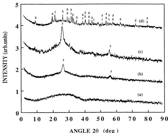
FIG. 2. X-ray-diffraction pattern at room temperature for (a) as-sputtered films of  $0.75\text{BiFeO}_3-0.125\text{ZnFe}_2\text{O}_4$  and for samples annealed at (b) 475 °C, (c) 525 °C, and (d) 775 °C. The high-temperature annealing leads to the precipitation of crystalline (1)  $\text{BiFeO}_3$ , (2)  $\gamma\text{-Fe}_2\text{O}_3$ , and (3)  $24\text{Bi}_2\text{O}_3 \cdot \text{ZnO}$  phases.
