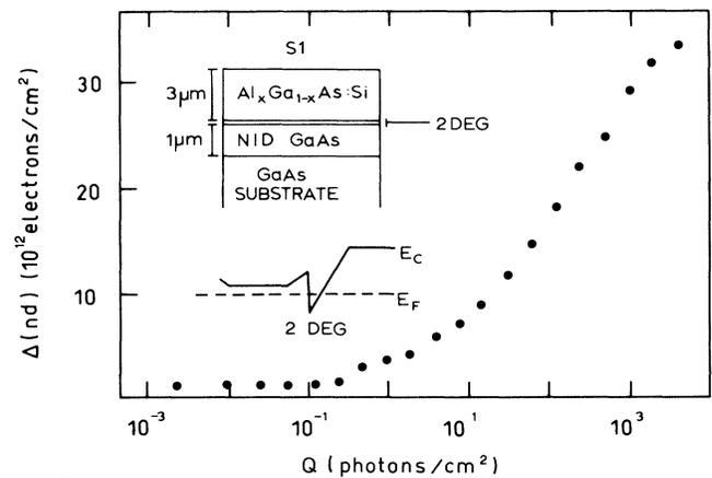
FIG. 4. Sheet persisting electron density  $\Delta(nd)$  vs cumulative photon dose  $Q$  (reduced with respect to a reference value) for layered sample *S1*.
