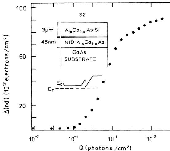
FIG. 5. Dependence of sheet electron density  $\Delta(nd)$  upon photon dose  $Q$  for sample S2.
