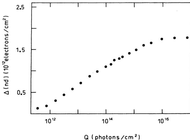
FIG. 3. Dependence of sheet electron density  $\Delta(nd)$  upon photon dose  $Q$ , according to Ref. 3, for an *N*-type GaAs epitaxial layer with  $d = 300 \text{ nm}$ , at 32 K.
