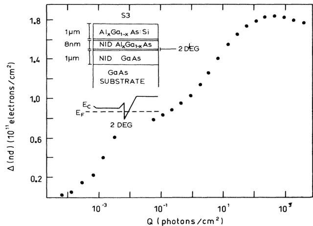
FIG. 6. Sheet electron concentration  $\Delta(nd)$  as a function of photon dose  $Q$  for sample S3.
