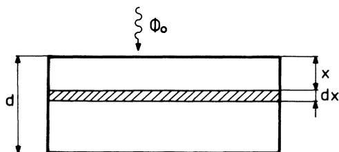
FIG. 1. Generic structure for the observation of the PP effect. The epitaxial layer of total depth *d* is exposed to a uniform photon flux *φ*<sub>0</sub>.
