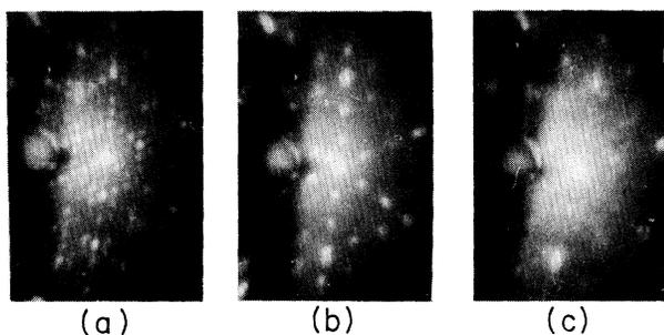
FIG. 1. LEED patterns of (a) a clean Si(111)7×7 surface; (b) a Si(111) surface after Na-induced 3×1 reconstruction; (c) a Si(111) surface after desorption of Na from (b) by heating to 920 K.  $E_p = 90$  eV.
