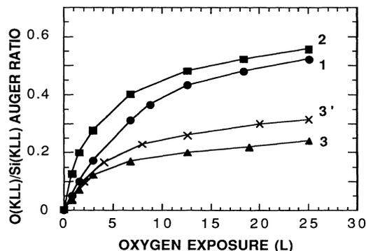
FIG. 3. Oxygen uptake curves for oxygen adsorption on 1, a clean Si(111) $7 \times 7$  surface; 2, a 0.1 Na/Si(111) $7 \times 7$  surface; 3, a "perfect" 0.1Na/Si(111) $3 \times 1$  surface; 3', an "imperfect" 0.1 Na/Si(111) $3 \times 1$  surface.  $T_a = 300$  K.
