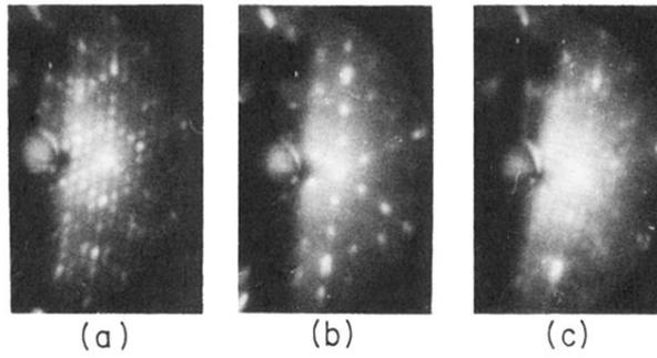
FIG. 1. LEED patterns of (a) a clean Si(111)7×7 surface; (b) a Si(111) surface after Na-induced 3×1 reconstruction; (c) a Si(111) surface after desorption of Na from (b) by heating to 920 K.  $E_p = 90$  eV.
