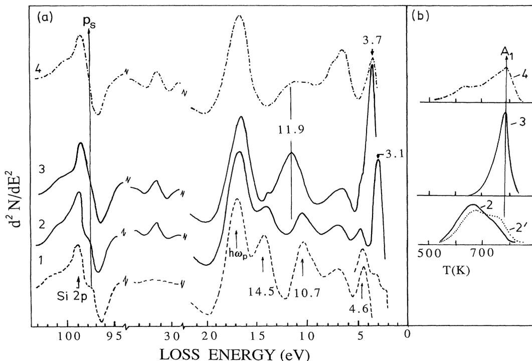
FIG. 2. (a) EEL spectra of 1, a clean Si(111)7×7 surface; 2, a 0.1 Na/Si(111)7×7 surface; 3, a 0.1Na/Si(111)3×1 surface; 4, after exposure of the 0.1 Na/Si(111)3×1 surface to 3000-L oxygen at 300 K.  $E_p = 90$  and 250 eV. (b) Na TPD spectra from 2, 0.1Na/Si(111)7×7; 2', 0.1Na+0.3O/Si(111)7×7; 3', 0.1Na/Si(111)3×1; 4, 0.1Na+0.3O/Si(111)3×1.  $dT/dt = 2$  K/s.
