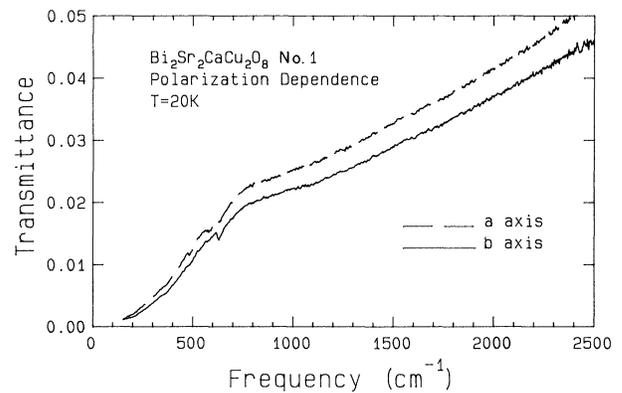
FIG. 3 Polarized transmittance of a single-domain  $\text{Bi}_2\text{Sr}_2\text{CaCu}_2\text{O}_8$  sample at 20 K.
