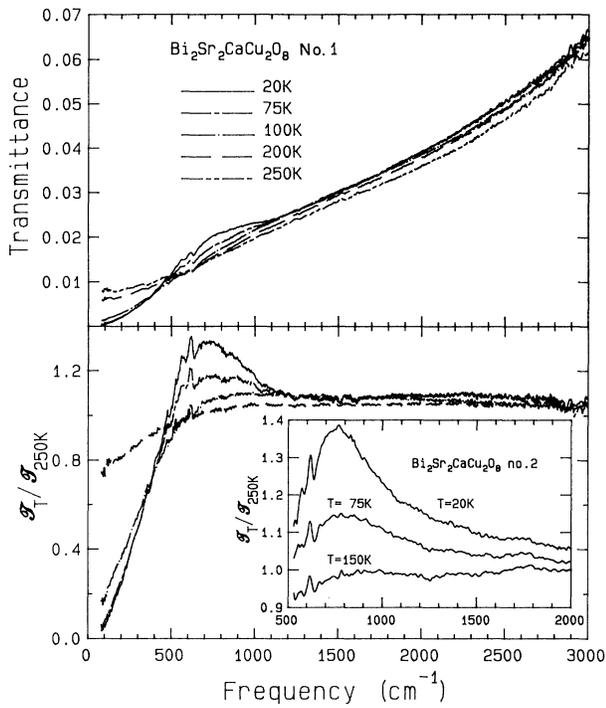
FIG. 1 Upper panel: transmittance spectra of a 1350-Å thick  $\text{Bi}_2\text{Sr}_2\text{CaCu}_2\text{O}_8$  sample at temperatures between 20 K and 250 K. Lower panel: The ratio,  $T_T/T_{250\text{K}}$ , of the spectra shown above. The inset shows  $T_T/T_{250\text{K}}$  for a second 2:2:1:2 sample.
