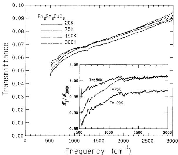
FIG. 2 Transmittance of a nonsuperconducting  $\text{Bi}_2\text{Sr}_2\text{CuO}_6$  sample at temperatures between 20 K and 300 K. The inset shows  $T_T/T_{300\text{K}}$ .
