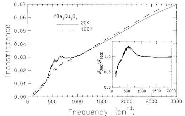
FIG. 4 Transmittance of a 1350-Å thick  $\text{YBa}_2\text{Cu}_3\text{O}_{7-\delta}$  film at 20 and 100 K, calculated from the Kramers-Kronig derived optical constants of Ref. 6. The inset shows  $\mathcal{T}_{20\text{ K}}/\mathcal{T}_{100\text{ K}}$ .
