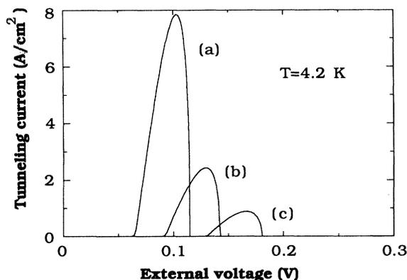
FIG. 3. The effective of  $\pm 10.86$ -Å change in barrier and well widths on  $I$ - $V$  spectra. (a) 74.08-Å barrier/66.92-Å well/74.08-Å barrier; (b) 85-Å barrier/56-Å well/85-Å barrier; (c) 95.92-Å barrier/45.08-Å well/95.92-Å barrier.
