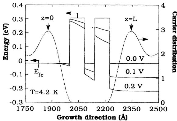
FIG. 1. Band diagrams (solid lines, 0.0-, 0.1-, and 0.2-V bias) and carrier distribution (dotted line,  $\times 10^{17} \text{ cm}^{-3}$ ) at thermal equilibrium, calculated at  $T=4.2 \text{ K}$ . The  $z=0$  and  $L$  are where the electrons are emitted and collected, respectively.  $E_{fe}$  is the quasi-Fermi level position in the emitter region.
