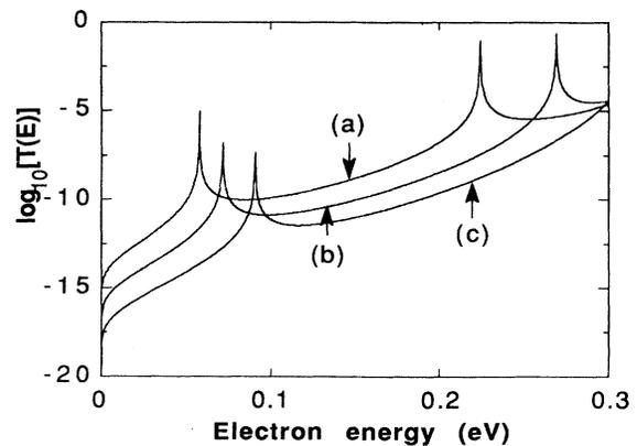
FIG. 2. Tunneling probability  $T(E)$  as a function of incident electron energy at zero bias. (a)  $74.08\text{-\AA}$  barrier/ $66.92\text{-\AA}$  well/ $74.08\text{-\AA}$  barrier; (b)  $85\text{-\AA}$  barrier/ $56\text{-\AA}$  well/ $85\text{-\AA}$  barrier; (c)  $95.92\text{-\AA}$  barrier/ $45.08\text{-\AA}$  well/ $95.92\text{-\AA}$  barrier.
