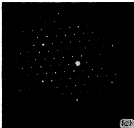
FIG. 3. (a) A representative electron micrograph of a rapidly solidified alloy showing an icosahedral grain in contact with the crystalline grains, (b) SAD pattern showing a superimposition of reflections from the i phase with threefold zone axis and \langle 111 \rangle bcc metastable phase, and (c) SAD pattern corresponding to \langle 111 \rangle zone axis of the bcc phase.
