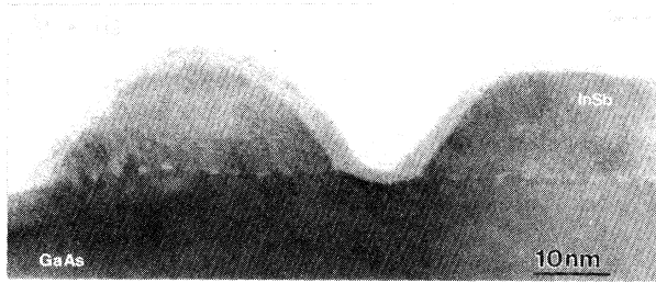
FIG. 5. Cross-sectional transmission electron micrograph showing a lattice image of a 13-nm-high InSb island on a GaAs surface. The zone axis of the image is (110) and fringes in the image are (111) planes. The bright points along the heterojunction indicate the presence of misfit dislocations. The dislocations are pure edge type with an average spacing of one every seven (111) planes.
