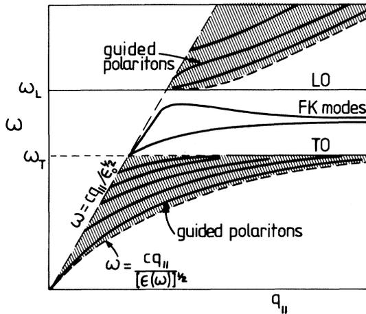
FIG. 3. Surface and guided polariton dispersion in a slab.  $\epsilon(\omega)$  is the frequency-dependent dielectric constant  $\epsilon(\omega) \rightarrow \epsilon_s(\omega=0)$ ,  $\epsilon(\omega) \rightarrow \epsilon_\infty(\omega \rightarrow \infty)$ . Note that the whole span of  $q_{||}$  depicted is small compared with typical wave vectors involved in the electron-phonon interaction.
