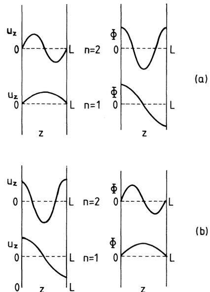
FIG. 1. Mode patterns for  $n=1$  and  $n=2$ : (a) HD and linear chain models, (b) EM model.
