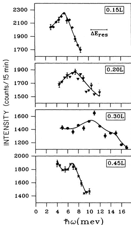
FIG. 2. Constant- $Q$  scans of the longitudinal modes along a fivefold axis for a fixed final energy of 30.5 meV. Lines are intended as a guide to the eye. The horizontal bar denotes the energy resolution for this configuration.
