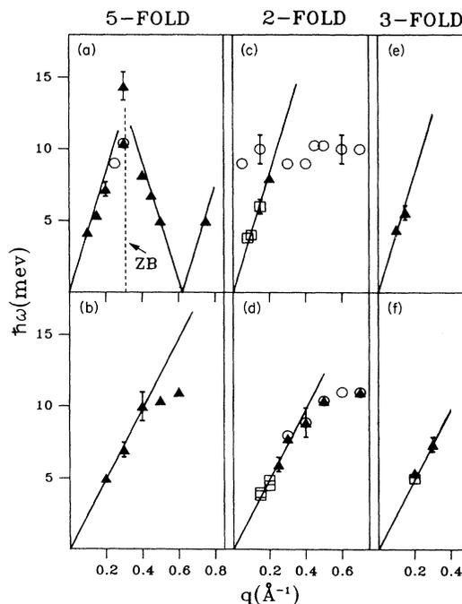
FIG. 3. The measured dispersion relations for fivefold (a) longitudinal and (b) transverse modes; twofold (c) longitudinal and (d) transverse modes; and threefold (e) longitudinal and (f) transverse modes. Circles, triangles, and squares denote measurements made at fixed final neutron energies of 42, 30.5, and 14.7 meV, respectively. The solid lines represent the initial slope of the dispersion curves calculated from measured sound velocities as described in the text.
