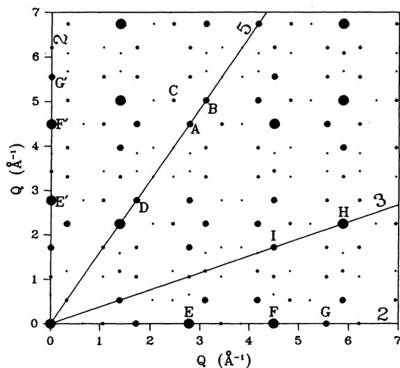
FIG. 1. A schematic of the twofold plane. Axes are labeled as the twofold, threefold, and fivefold directions. Letters denote the "zone-centers" from which inelastic scattering measurements were made.
