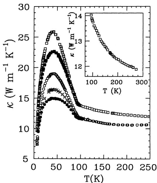
FIG. 1. Thermal conductivity for samples 1 and 2. Open and solid squares show sample 1 in zero field and at 1.5 T, respectively. Open circles, stars, and solid circles stand for sample 2 in zero field, 2, and 6 T, respectively. The inset presents a magnified plot of  $\kappa(T)$  at  $T > T_c$  for sample 1.
