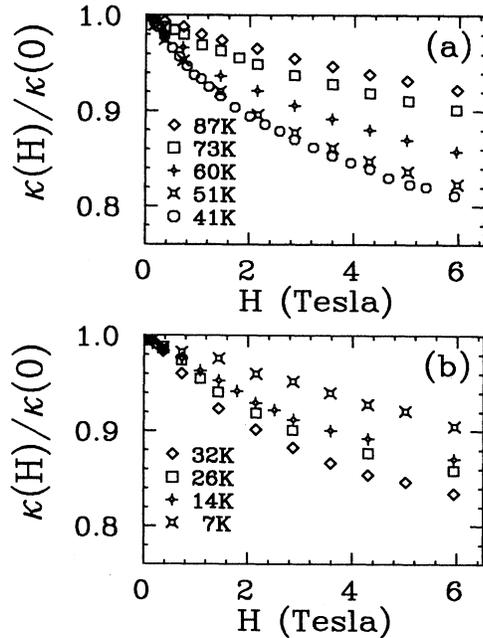
FIG. 2. (a),(b) Field dependence of the thermal conductivity at different temperatures for sample 2 (increasing field applied perpendicular to the  $a$ - $b$  plane).
