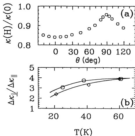
FIG. 4. (a) Angular dependence of the thermal conductivity for sample 1 at 41 K and  $H=1.5$  T.  $\theta$  is the angle between the magnetic field and the  $c$  axis of the crystal. (b) Anisotropy  $\Delta\kappa_{\perp}/\Delta\kappa_{\parallel}$  (defined in the text) for specimen 1 at 1.5 T (circles) and specimen 2 at 3 T (diamonds). The solid line is a guide to the eye.
