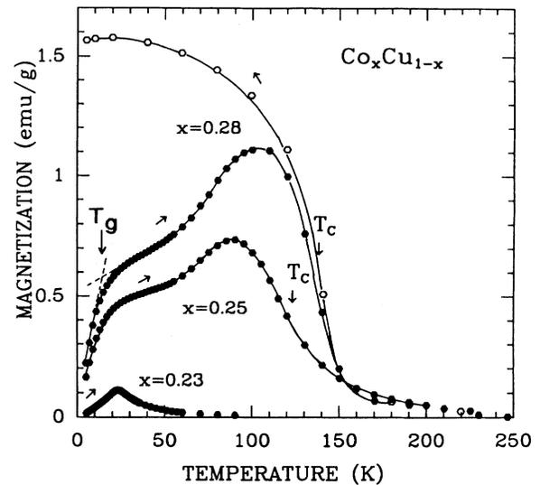
FIG. 5. Typical zero-field-cooled magnetization curves (solid circles) for  $\text{Co}_x\text{Cu}_{1-x}$  in reentrant regime, with  $H_{\text{ext}}=10$  G. The field cooled data is also shown for  $x=0.28$  (open circles).
