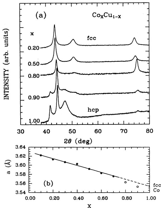
FIG. 1. (a) X-ray spectra of sputtered  $\text{Co}_x\text{Cu}_{1-x}$  alloys. The Co hcp phase appears only above  $x=0.80$ . (b) Crystalline lattice spacing  $a$  obtained from fcc spectra as a function of  $x$ .
