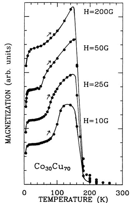
FIG. 6. Zero-field-cooled Magnetization of  $\text{Co}_{30}\text{Cu}_{70}$  as a function of temperature, for different values of the external field  $H_{\text{ext}}$ .
