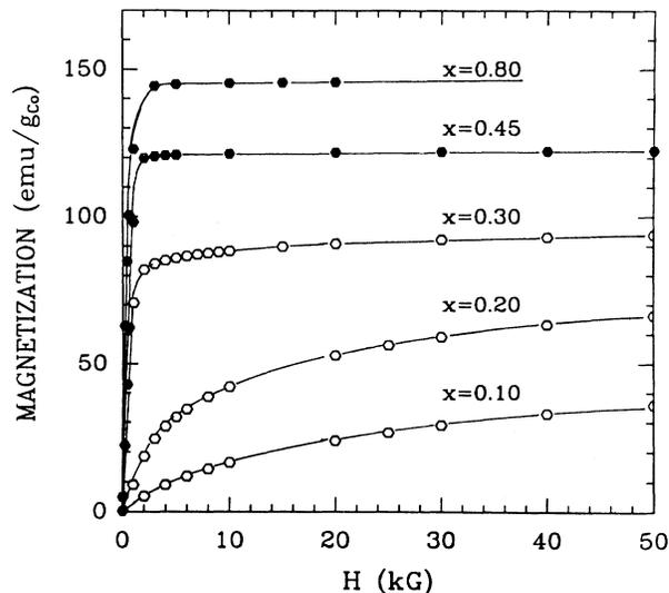
FIG. 2. Magnetization versus applied field for  $\text{Co}_x\text{Cu}_{1-x}$ , in units of emu per gram of Co, at  $T=5 \text{ K}$ . Full saturation is not reached at  $H=50 \text{ kG}$  for  $x \leq 0.30$  (open circles).
