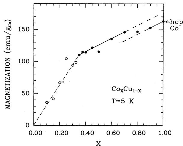
FIG. 3. Solid circles: Saturation magnetization of sputtered  $\text{Co}_x\text{Cu}_{1-x}$  alloys as a function of  $x$ , in units of emu/g of Co. Open circles: Magnetization under an applied field of 50 kG.
