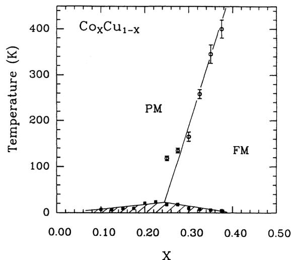
FIG. 7. Magnetic phase diagram of fcc  $\text{Co}_x\text{Cu}_{1-x}$  showing paramagnetic (PM), ferromagnetic (FM) and spin-glass (shaded area) phases.
