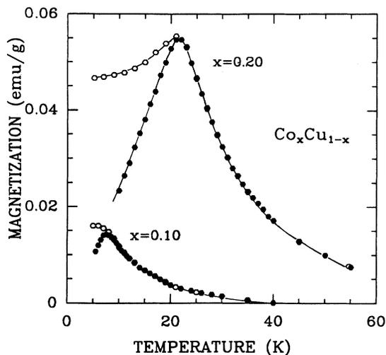
FIG. 4. Typical zero-field-cooled (solid circles) and field-cooled (open circles) magnetization curves for  $\text{Co}_x\text{Cu}_{1-x}$  in spin-glass regime, with  $H_{\text{ext}}=50$  G and  $10$  G for  $x=0.10$  and  $x=0.20$ , respectively.
