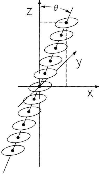
FIG. 4. Aligned stack of 2D pancake vortices tilted at angle  $\theta$  relative to the  $z$  axis.
