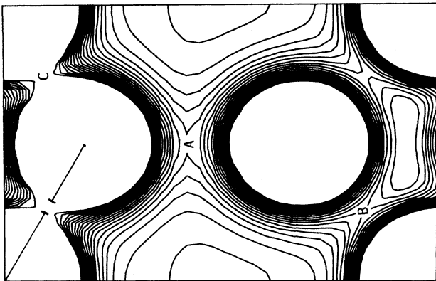
FIG. 12. Contours of equal charge density in a \langle 100 \rangle plane through two oxygen (center) and four zirconium (corners) atoms for a tetragonal zirconia.
