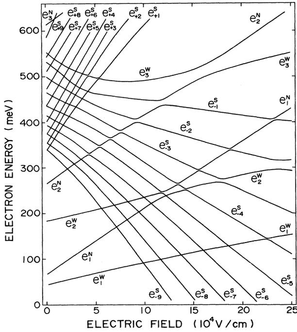
FIG. 2. Calculated electron eigenenergies of the 100- and 80-Å-thick GaAs quantum wells separated by an 8-Å AlAs barrier layer and sandwiched by nine alternating layers of 8-Å-thick AlAs and 25-Å-thick GaAs as a function of the electric field.
