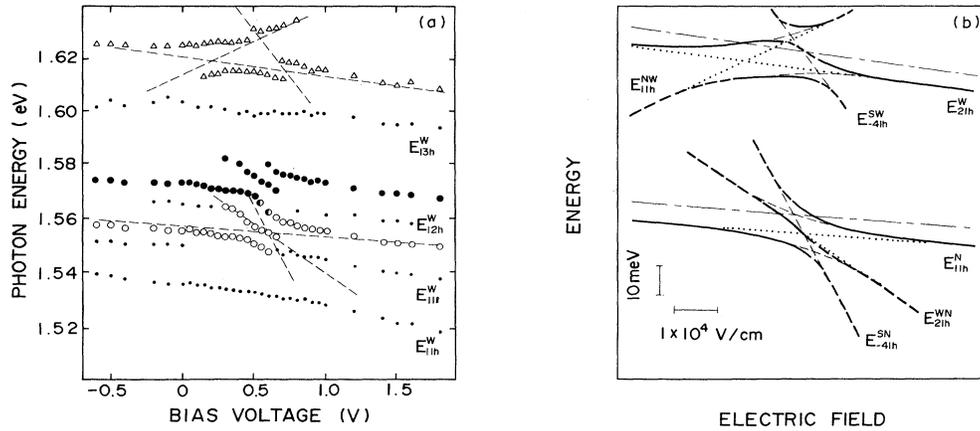
FIG. 3. (a) Absorption peak energies as a function of the external bias voltage  $V_{ex}$ . The data were taken from the photocurrent spectra measured at 77 K. (b) A graphical explanation of the experimental results according to the mixing between the three optical transitions. Two dotted lines and a thin dashed straight line in (b) correspond to the three dashed lines in (a). For simplicity, the illustration for the solid circle group is not given.
