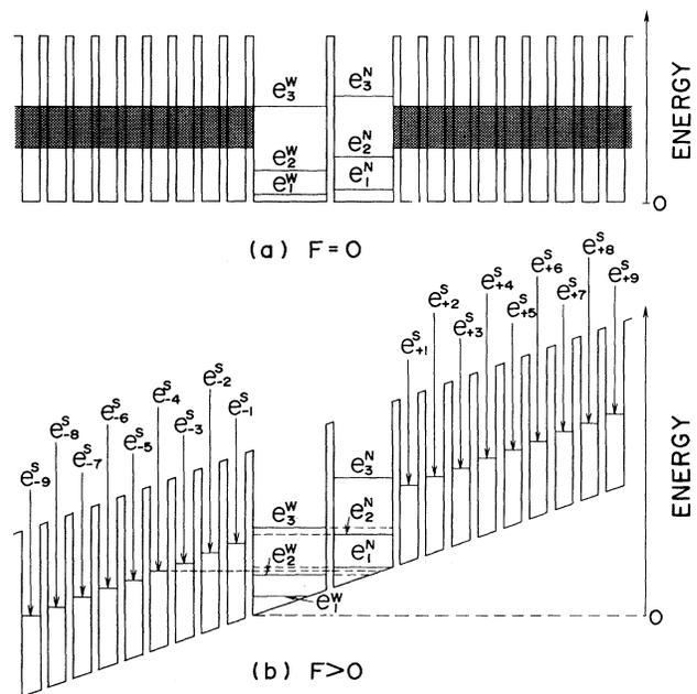
FIG. 1. Schematically illustrated potential profiles of the conduction bands of a GaAs asymmetric potential coupled quantum well confined by the AlAs-GaAs superlattices in different electric fields  $F$ : (a)  $F=0$ ; (b)  $F>0$ .
