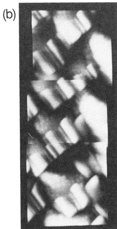
FIG. 3. Mosaic images of (a) 5-ML and (b) 10-ML Ag depositions showing the formation of nanocrystallites orientated along [1\bar{1}0] and [001] . Each image used in the mosaic is \sim 425 \times 425 \text{ \AA}^2 .
