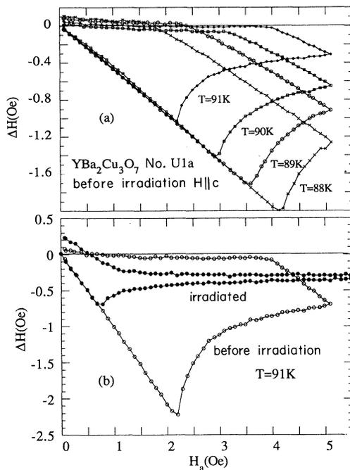
FIG. 3. (a) Typical magnetization loops for sample U1a before irradiation. Note the almost-zero magnetization of the descending branch. (b) Magnetization loops recorded at 91 K for sample U1a before and after electron irradiation. The initial Meissner slope was normalized to  $-1$ , by dividing each  $M$  value by apparent value of initial slope, in order to account for small difference of Hall probe position in two runs.
