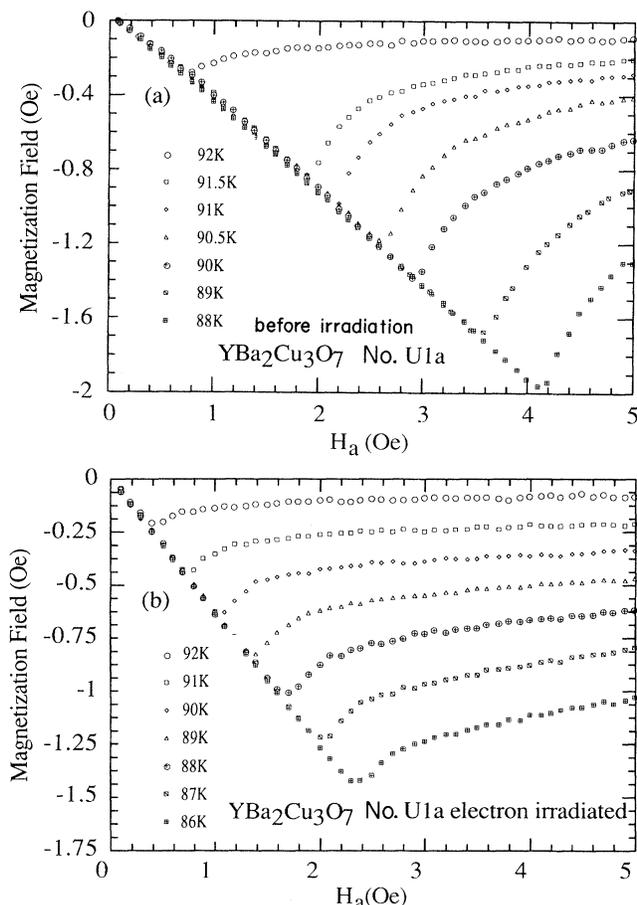
FIG. 1. Magnetization curves for untwinned Y-Ba-Cu-O, sample U1a, at the indicated temperatures (a) before and (b) after irradiation.
