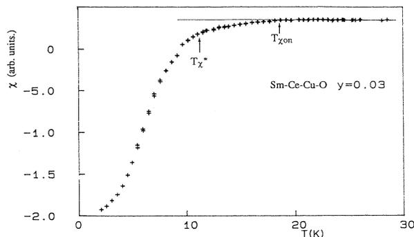
FIG. 9. Field-cooled magnetic susceptibility of  $\text{Sm}_{1.85}\text{Ce}_{0.15}\text{CuO}_{3.97}$  sample as a function of temperature measured under 28 Oe applied field. Moderate signal variation below  $T_{\chi\text{on}}$  becomes much steeper at  $T_{\chi}^*$ .
