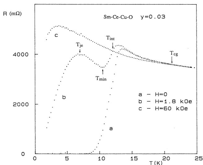
FIG. 4. Resistance of  $\text{Sm}_{1.85}\text{Ce}_{0.15}\text{CuO}_{3.97}$  sample as a function of temperature under different applied magnetic fields. The measuring current is  $100 \mu\text{A}$ . Double-peak transition including the resistance enhancement below  $T_{cg}$  is pronounced under  $H=1.8 \text{ kOe}$ .
