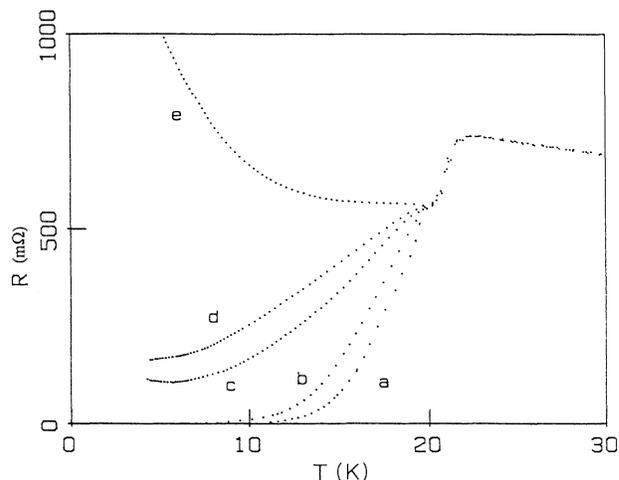
FIG. 2. Resistance of  $\text{Sm}_{1.85}\text{Ce}_{0.15}\text{CuO}_{3.98}$  sample as a function of temperature measured with different current levels at zero applied field. (a) 1 mA, (b) 2 mA, (c) 4 mA, (d) 5 mA, and (e) 10 mA. An initial current-independent resistance drop can be related to the intragranular transition, when the current-dependent stage is a property of intergranular boundaries.
