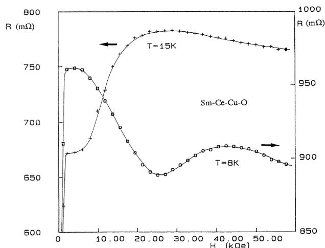
FIG. 6. Resistance of  $\text{Sm}_{1.85}\text{Ce}_{0.15}\text{CuO}_{3.98}$  sample as a function of applied magnetic field at two temperatures 8 and 15 K. The measuring current is  $100 \mu\text{A}$ . Double-peak magnetoresistance transition is seen at 8 K.
