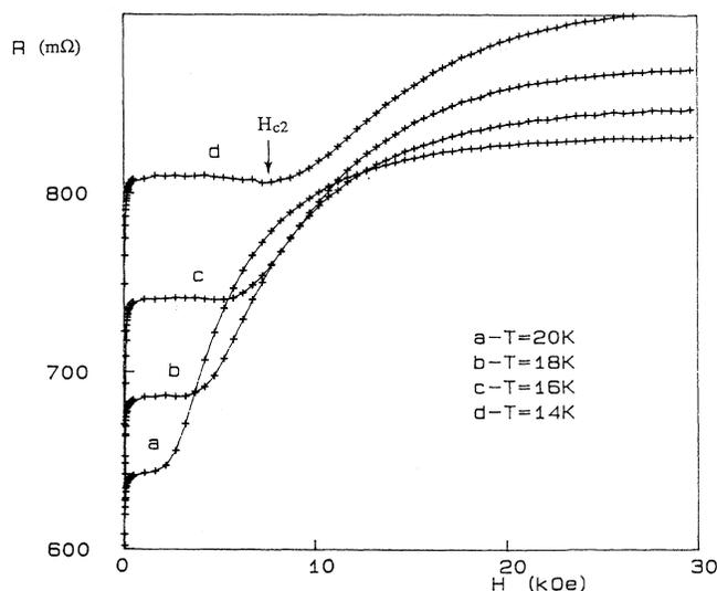
FIG. 11. Low-field magnetoresistance of  $\text{Sm}_{1.85}\text{Ce}_{0.15}\text{CuO}_{3.98}$  sample measured at several temperatures in the vicinity of  $T_{\text{min}}$ . Identification of  $H_{c2}$  is discussed in the text.
