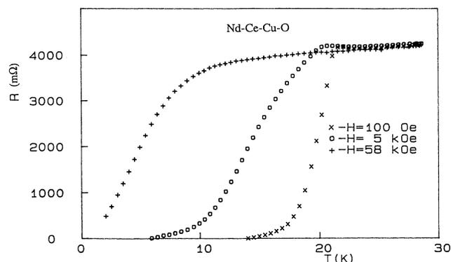
FIG. 5. Resistance of  $\text{Nd}_{1.85}\text{Ce}_{0.15}\text{CuO}_{3.98}$  sample as a function of temperature under different applied magnetic fields. The measuring current is  $100 \mu\text{A}$ . Enhancement of resistance below  $T_{cg}$  measured under low field is observed also in this sample with a metal-like normal-state behavior ( $dR/dT > 0$ ).
