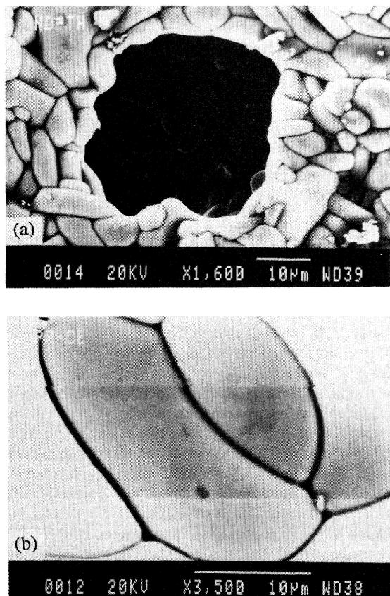
FIG. 1. SEM micrographs of (a) Nd-Th-Cu-O and (b) Pr-Ce-Cu-O samples. The grains are large and tightly packed.
