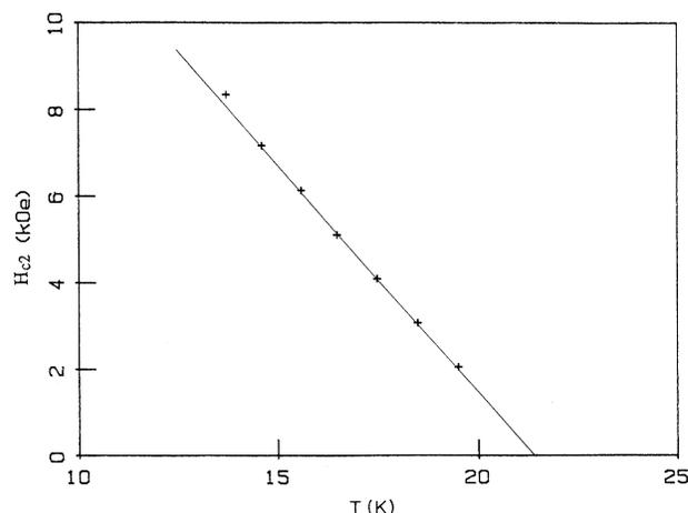
FIG. 12. Upper critical field  $H_{c2}$  in direction parallel to the  $c$  axis of  $\text{Sm}_{1.85}\text{Ce}_{0.15}\text{CuO}_{3.98}$  as a function of temperature.
