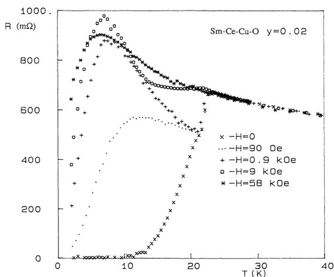
FIG. 3. Resistance of  $\text{Sm}_{1.85}\text{Ce}_{0.15}\text{CuO}_{3.98}$  sample as a function of temperature under different applied magnetic fields. The measured current is 100  $\mu\text{A}$ . Nonmonotonic resistive transition is emphasized under  $H = 0.9 \text{ kOe}$ .
