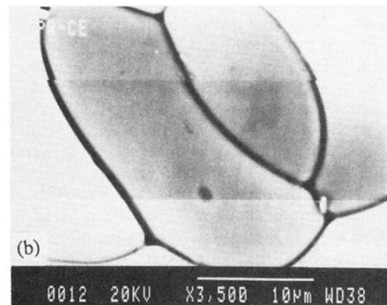
FIG. 1. SEM micrographs of (a) Nd-Th-Cu-O and (b) Pr-Ce-Cu-O samples. The grains are large and tightly packed.
