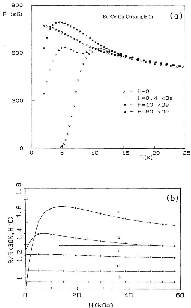
FIG. 7. (a) Resistance of a large  $\text{Eu}_{1.85}\text{Ce}_{0.15}\text{CuO}_{3.98}$  sample as a function of temperature under different applied magnetic fields. The measuring current is  $100 \mu\text{A}$ . (b) Normalized resistance of a large  $\text{Eu}_{1.85}\text{Ce}_{0.15}\text{CuO}_{3.98}$  sample as a function of applied magnetic field at temperatures: (a) 5 K, (b) 10 K, (c) 14.5 K, (d) 24 K, and (e) 33 K.
