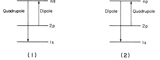
FIG. 5. Two processes allowed in a two-photon transition from the 2p to 1s state.
