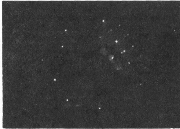
FIG. 2. LEED pattern of the clean reconstructed Mo(001) surface at 100 K, obtained with the in situ LEED system at \approx 250 eV electron energy and close to normal incidence. The LEED screen is partly obscured by the target holder. Diffraction from predominantly one of the two possible domains of the periodic lattice distortion is to be seen. The He diffraction of Fig. 1 was measured in the azimuth of the visible doublet of superstructure spots.
