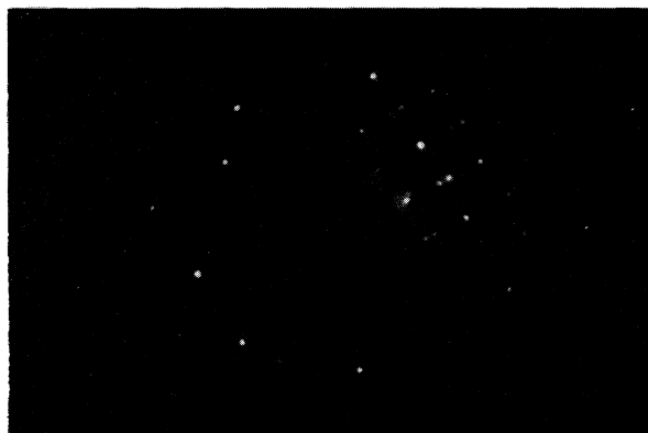
FIG. 2. LEED pattern of the clean reconstructed Mo(001) surface at 100 K, obtained with the in situ LEED system at \approx 250 eV electron energy and close to normal incidence. The LEED screen is partly obscured by the target holder. Diffraction from predominantly one of the two possible domains of the periodic lattice distortion is to be seen. The He diffraction of Fig. 1 was measured in the azimuth of the visible doublet of superstructure spots.
