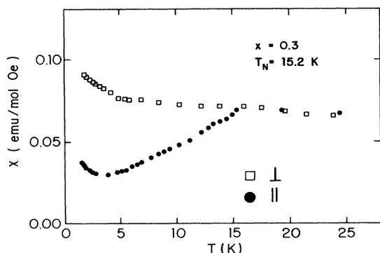
FIG. 1. Zero-field magnetic susceptibility parallel and perpendicular to the easy axis for  $K_2Fe(Cl_{0.7}Br_{0.3})_5 \cdot H_2O$  as a function of the temperature.
