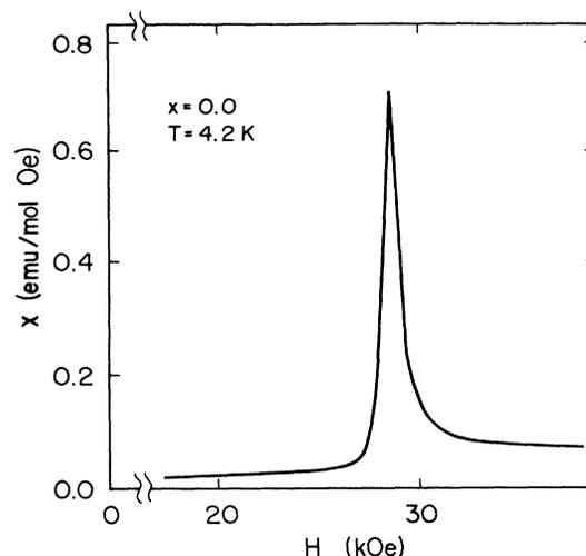
FIG. 2. Magnetic susceptibility as a function of the applied field for  $K_2FeCl_5 \cdot H_2O$ . The peak corresponds to the first-order AF-SF transition.
