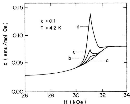
FIG. 3. Susceptibility as a function of the external applied field in the region of the AF-SF transition in  $K_2Fe(Cl_{0.9}Br_{0.1})_5 \cdot H_2O$  for different peak-to-peak values of the modulation field: (a) 55 Oe, (b) 70 Oe, (c) 85 Oe, and (d) 110 Oe.
