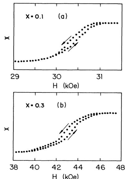
FIG. 5. Susceptibility ( $\chi$ ) versus applied field ( $H$ ) for increasing and decreasing  $H$ . The modulation field was 1 Oe and the temperature 2.0 K. Note the different scale of the field axis. The curves were taken at very slow  $dH/dt$ .
