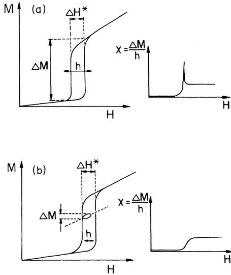
FIG. 6. Schematic representation of the magnetization  $M$  and susceptibility at the first-order AF-SF transition when hysteresis  $\Delta H^*$  is present: (a) when  $h > \Delta H^*$  the measured susceptibility  $\Delta M/h$  shows a sharp peak at the transition. (b) when  $h < \Delta H^*$  the measured  $\Delta M/h$  is given by the slope of the minor hysteresis loop.
