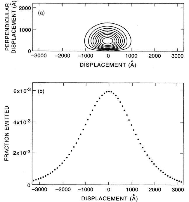
FIG. 6. (a) Positron density contours for 5 keV positrons implanted in a 2200 Å-thick Ni crystal. (b) Positron emission profile from the surface opposite the point of implantation using  $D_+ = 1.6 \text{ cm}^2 \text{ s}^{-1}$ ,  $\mathcal{R} = 0.7$ , and  $\tau_{\text{eff}} = 100 \text{ ps}$ . The profile is Gaussian shaped and the width is characterized by the standard deviation ( $\sigma$ ) of the Gaussian.
