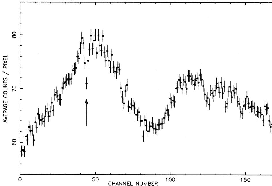
FIG. 2. A 36 pixel wide cut through a magnified ( $4400\times$ ) image of defect structures. From the FWHM of the cut through the sharp feature (indicated by the arrow), we determined the PRM resolution is  $2\Delta r = 800$  Å. One channel equals 355 Å.
