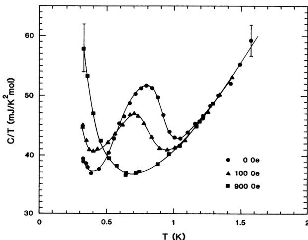
FIG. 1. Temperature dependence of the specific heat  $C$  divided by temperature  $T$  for a magnetic field parallel to the  $b^*$  axis for  $\alpha$ -(ET)<sub>2</sub>(NH<sub>4</sub>)Hg(SCN)<sub>4</sub>.
