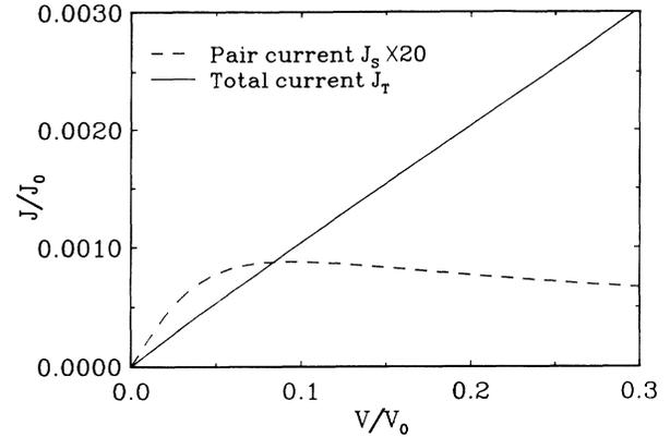
FIG. 3. Calculation of  $I(V)$  using theory of Geshkenbein and Sokol [Eq. (16) of Ref. 10] and parameter values  $D=0.01$ ,  $u=12$ , and  $T=4.48$  K appropriate to the pair-field susceptibility regime, in which small excess currents are observed. Similar curves are reported in Refs. 4 and 5.
