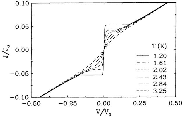
FIG. 1. Calculated  $I(V)$  curves obtained from the theory of Geshkenbein and Sokol [Eq. (16) of Ref. 10] using parameter values  $D=0.2$ ,  $T_{cs}=4.48$  K, and  $u=12$  (see text), appropriate to Ta point-contact tunnel junctions on Mo or  $UBe_{13}$ . Current and voltage scales normalized as in Ref. 11.
