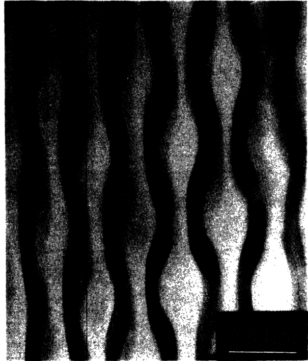
FIG. 3. Enlarged TEM view of a well-developed domain of oscillations ( U_\infty = 0.10 , V = 5.2 cm/s).
