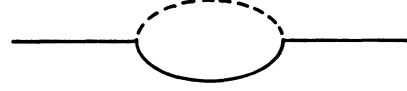
FIG. 1. O(g) self-energy correction to the electron propagator. Solid lines denote electrons while the dashed line denotes a phonon.
