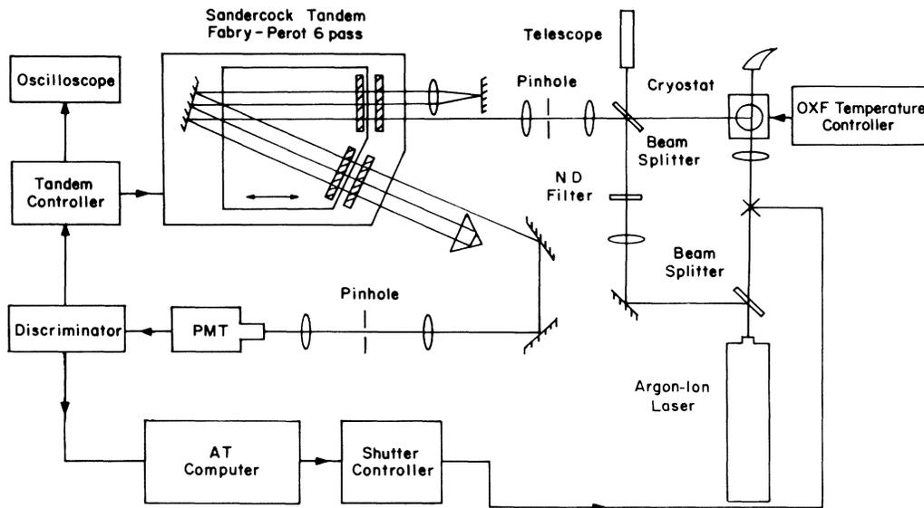
FIG. 1. Schematic illustration of the CCNY six-pass tandem interferometer Brillouin scattering apparatus. (ND denotes neutral density filter.)
