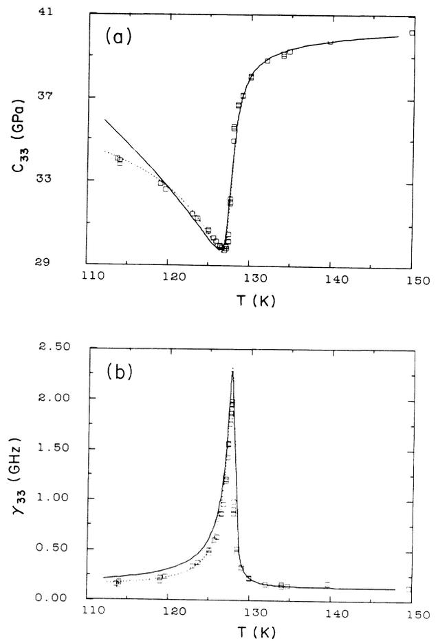
FIG. 8. Same as Fig. 7, but with the coefficients adjusted to simultaneously produce a best fit to both (a)  $C'_{33}(\omega)$  and (b)  $\gamma_{33}(\omega)$ . The resulting adjusted values of the free-energy coefficients are listed in the third column of Table I. Note that fits are shown using either  $D=0$  (solid lines) or  $g_3=0$  (dashed lines) with the  $g_3=0$  fits giving better agreement.
