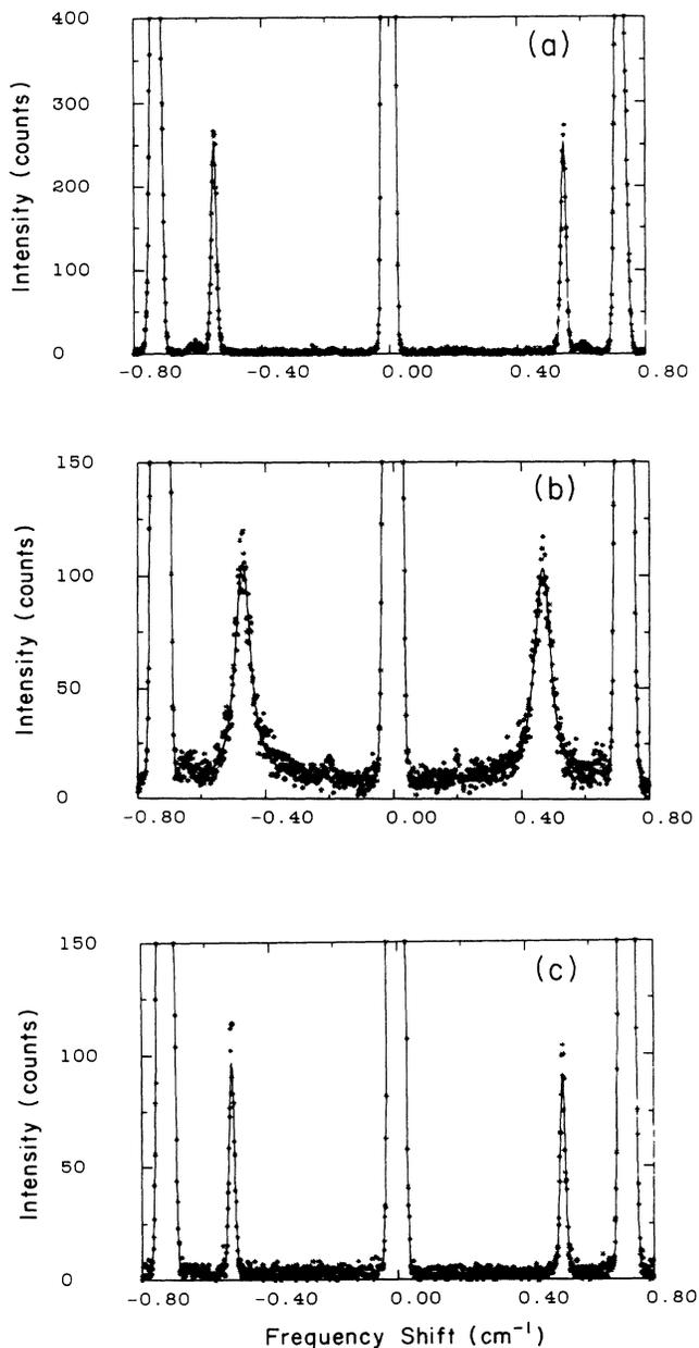
FIG. 2. Brillouin spectra of  $K_2SeO_4$  in the (a+c)[b,T](a-c) scattering geometry with  $\theta=90^\circ$  at (top to bottom) (a)  $T=300$  K, (b) 127.5 K, and (c) 81 K showing the  $C_{33}$  longitudinal-acoustic mode.
