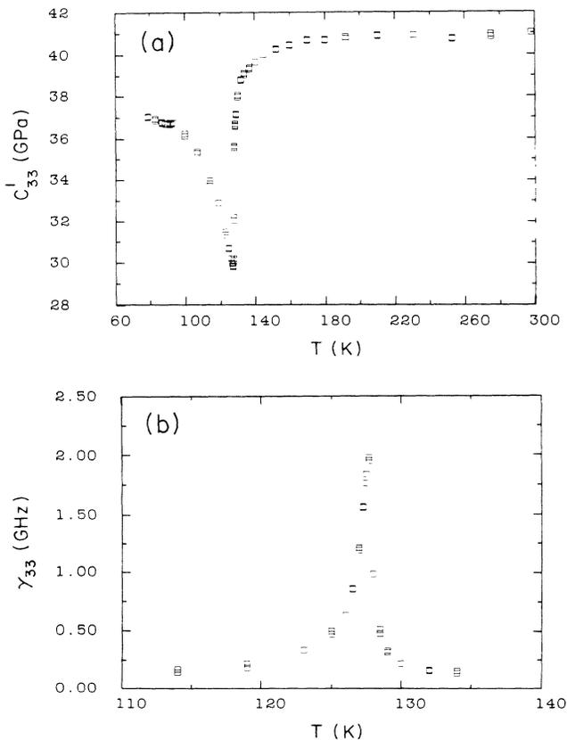
FIG. 5. Temperature dependences of (a)  $C'_{33}(\omega)$  and (b)  $\gamma_{33}(\omega)$  deduced from the  $90^\circ$  Brillouin-scattering data with damped harmonic-oscillator fits.
