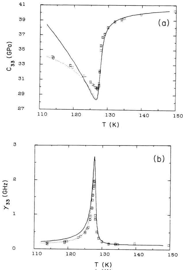
FIG. 7. Comparison of the  $90^\circ$  Billouin data of Fig. 5 with the theoretical predictions of Fig. 6 for (a)  $C'_{33}(\omega)$  and (b)  $\gamma_{33}(\omega)$ . Solid lines,  $D=0$ . Dotted lines,  $g_3=0$ . The theoretical fits include a phason gap  $\Omega_\phi(0)=160$  GHz. The free-energy coefficients used were those computed from the results of other experiments, listed in the second column of Table I.
