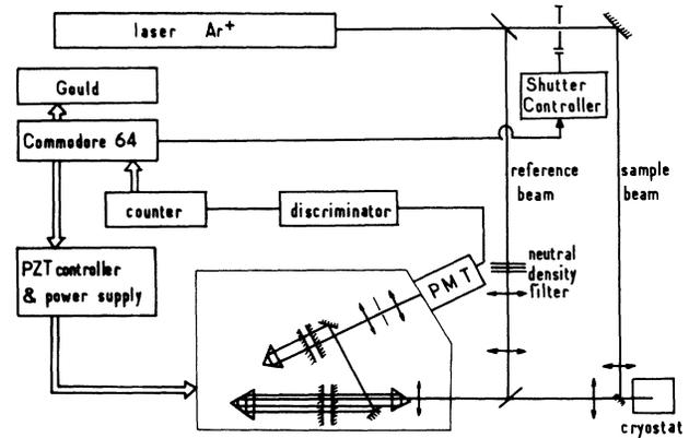
FIG. 3. Schematic illustration of the DRP six-pass tandem interferometer.
