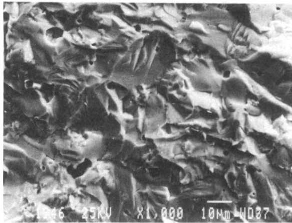
FIG. 2. Scanning electron micrograph of a cleaved surface for \text{Nd}_{1.85}\text{Ce}_{0.15}\text{CuO}_{4-y} (reduced). About 90% of the cleaved surface consists of transgranular cleavages and the other is voids and grain boundaries.
