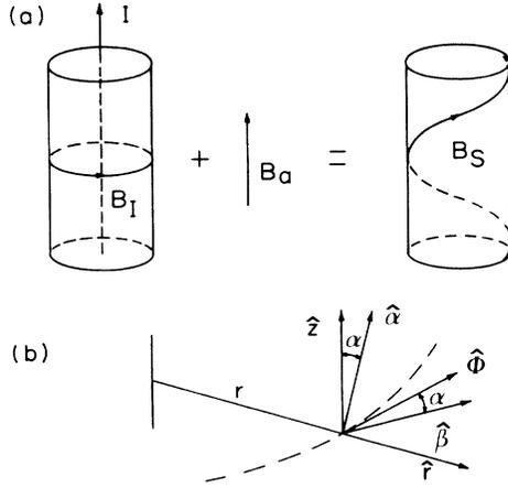
FIG. 1. (a) Experiment considered, and (b) local coordinates used in the calculations. Note that  $\hat{\alpha}$  and  $\hat{\beta}$  are perpendicular to  $\hat{r}$ .
