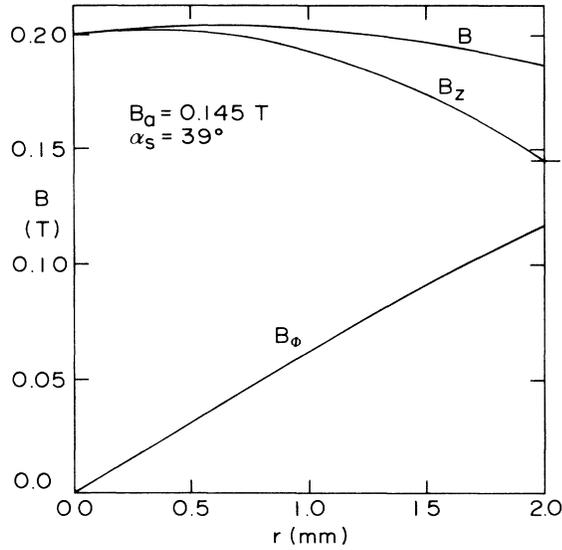
FIG. 3. Internal magnetic-field distribution at the critical current. In this case  $B_a=0.145$  T and  $J=J_c=9.367 \times 10^3$  A/cm<sup>2</sup>.
