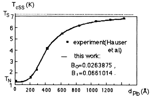
FIG. 3. Transition temperature of a Pb-Al lamina for a constant aluminum-film thickness of 4400 Å as a function of the lead-film thickness.
