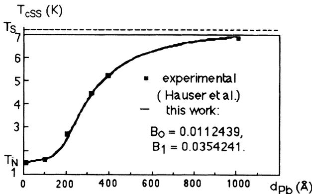
FIG. 2. Transition temperature for a Pb-Pb:2.9% Gd lamina with a constant Pb:2.9% Gd film of 5200 Å as a function of the lead-film thickness.
