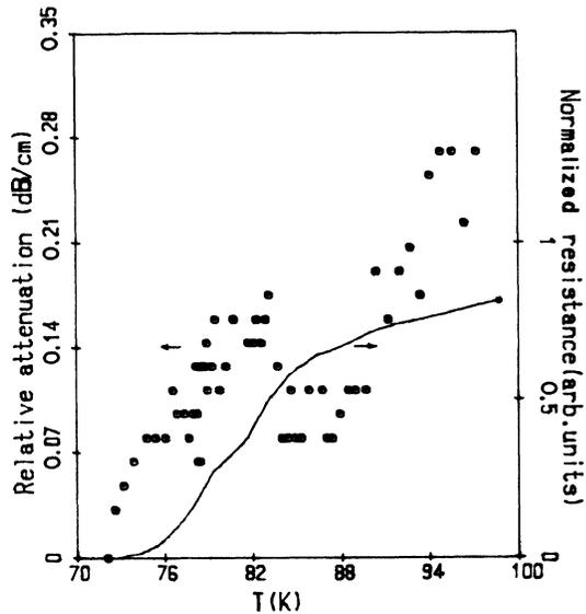
FIG. 12. Attenuation and normalized resistance vs temperature for sample 2. A weak peak near 82 K ( $T_{cmid}$ ) shows the characteristic of superconducting transition.  $f = 10$  MHz; longitudinal wave.
