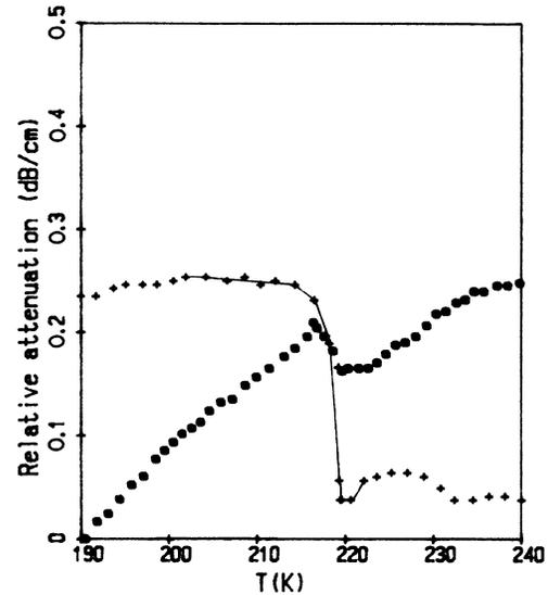
FIG. 3. Attenuation vs temperature for samples 3 (+) and 5 (o). Phase-transition-like anomalies for both of them are seen around 217 K.  $f = 10 \text{ MHz}$ ; longitudinal wave.
