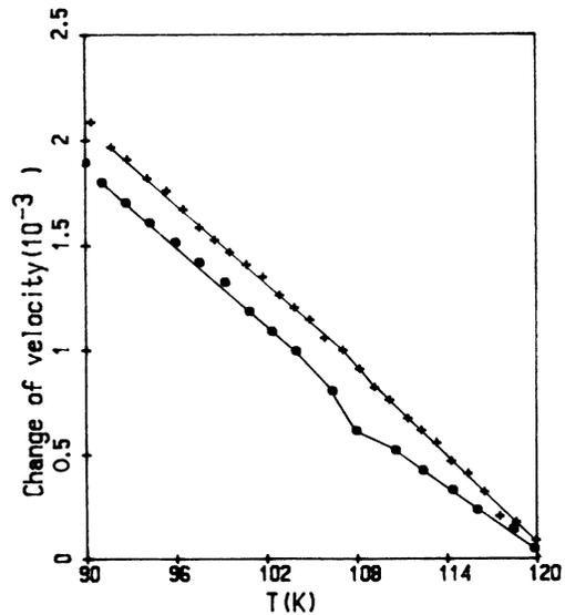
FIG. 11. Velocities of both longitudinal  $(\odot)$  and transverse  $(+)$  waves vs temperature for sample 5. Anomalies around 110 K indicate the pretransition in crystal lattice above  $T_c$ .  $f = 10$  MHz.
