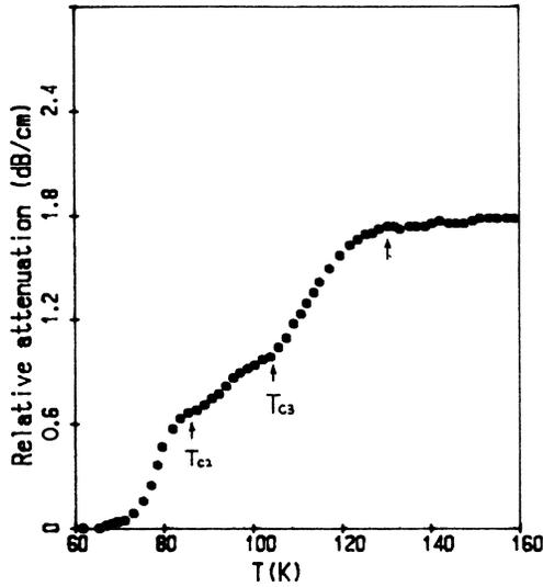
FIG. 8. Temperature dependence of attenuation for sample 1. Anomalies occur around 85, 106, and 130 K, respectively.  $f = 10$  MHz; longitudinal wave.
