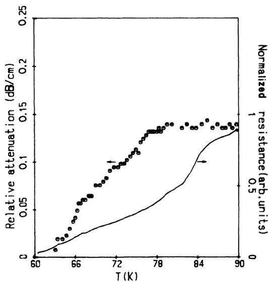
FIG. 13. Attenuation and normalized resistance vs temperature for sample 3. Rapid decrease after a short plateau is the anomaly in attenuation around  $T_c$ .  $f = 10$  MHz; longitudinal wave.
