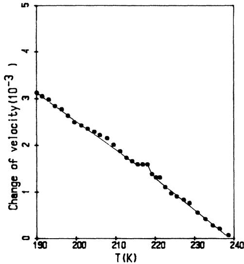
FIG. 4. Temperature dependence of velocity for sample 3. An anomaly around 217 K takes place and the slope of the curve below 217 K becomes smaller than that of above 217 K.  $f = 10$  MHz; longitudinal wave.
