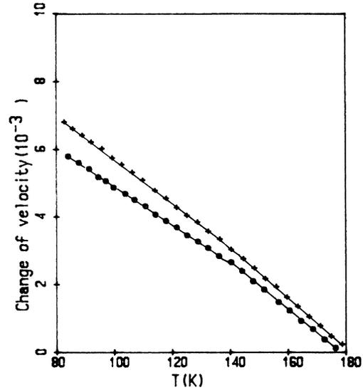
FIG. 10. Temperature dependence of velocities of both longitudinal,  $(\odot)$  and transverse  $(+)$  waves for sample 4. The slopes of both curves change at 140 K.
