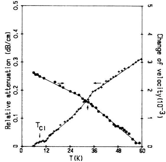
FIG. 16. Temperature dependence of velocity and attenuation for sample 4. Anomalies near 9 and 32 K are indicated by vertical arrows.  $f = 10$  MHz; longitudinal wave.
