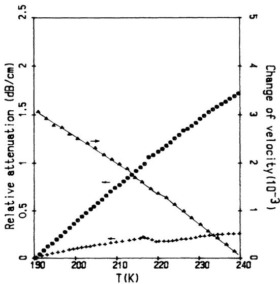
FIG. 5. Attenuation and velocity vs temperature for sample 5. A phase-transition-like anomaly appears around 217 K. Longitudinal ( $\blacktriangle$ ,  $+$ ) and transverse waves ( $\odot$ );  $f = 10$  MHz.
