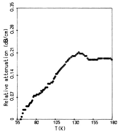
FIG. 7. Attenuation vs temperature for sample 3. Anomalies around 80 and 136 K are almost the same as those of sample 2.  $f = 10$  MHz; longitudinal wave.
