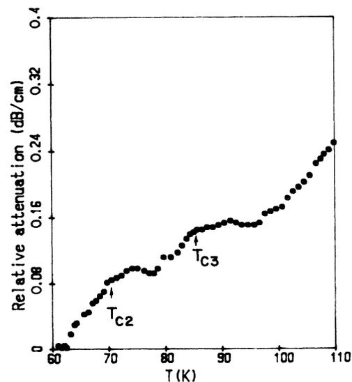
FIG. 15. Temperature dependence of attenuation for sample 5. Anomalies around 70 and 86 K are related to two superconducting transitions at these positions, respectively.  $f = 10$  MHz; transverse wave.
