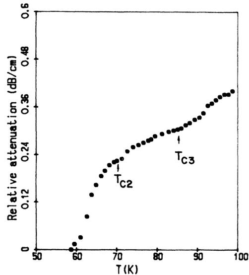
FIG. 14. Temperature dependence of attenuation for sample 5. Anomalies around 70 and 86 K are related to two superconducting transitions at these positions, respectively.  $f = 10$  MHz; longitudinal wave.
