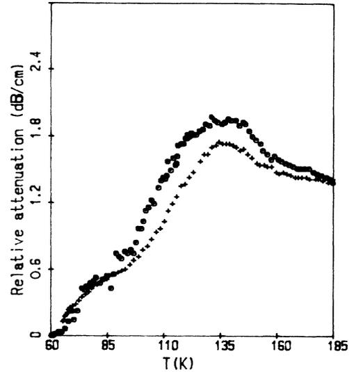
FIG. 6. Attenuation vs temperature for sample 2 in two warming up runs [ $\odot$  first run;  $+$  second run]. Stress reduction, anomalies near 81 and 136 K are seen clearly.  $f = 10$  MHz; longitudinal wave.
