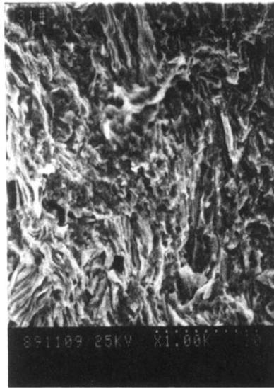
FIG. 2. SEM photograph for a sample hot pressed after sintering in air. The direction of pressure lies in horizon in this figure. The orientations of most granules (*c* axis) align the direction of pressure.
