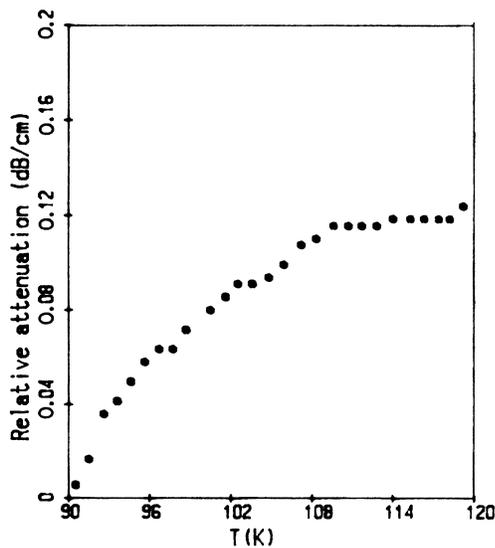
FIG. 9. Temperature dependence of attenuation for sample 5. An anomaly takes place at 110 K.  $f = 10$  MHz; longitudinal wave.
