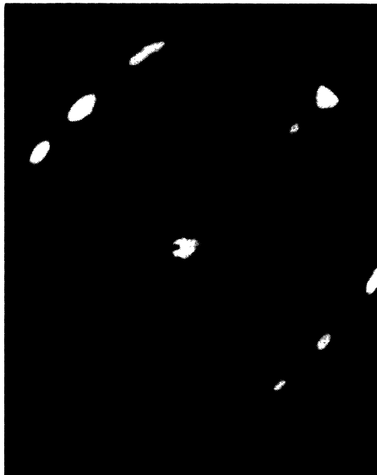
FIG. 2. LEED pattern observed for clean Ir(110) after annealing to 1400°C.
