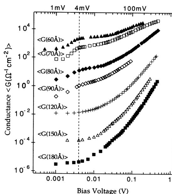
FIG. 2. Voltage dependence of the conductance of barriers with increasing thickness.
