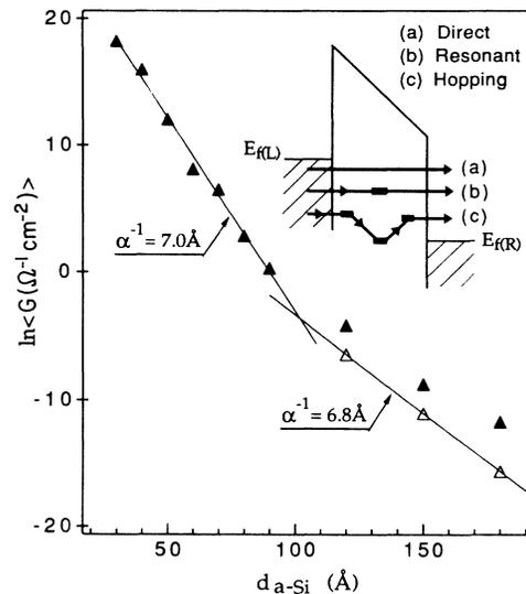
FIG. 1. Small-bias tunneling conductance as a function of barrier thickness. The solid triangles are measured data. The open triangles represent resonant-tunneling conductance corrected for that of hopping via a pair of localized states. Values of localization length  $\alpha^{-1}$  extracted from both direct and resonant-tunneling data are indicated. Inset shows three different tunneling processes.
