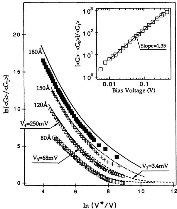
FIG. 3. Comparison between the experiment and the theory. The inset shows the normalized conductance as a function of bias voltage for  $d=70 \text{ \AA}$  barrier. The slope of the curve is the power exponent for hopping channels with two localized states.
